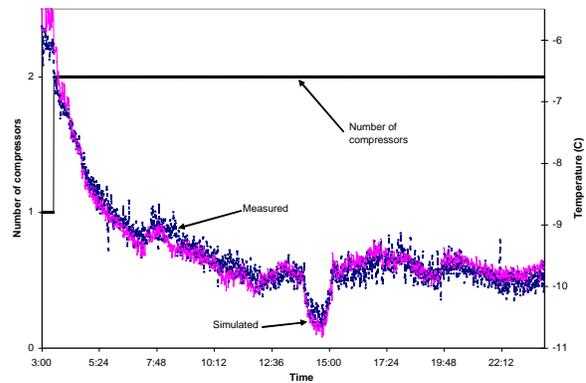
Figure 5: Open system simulation with given schedule. Measured vs simulated brine temperatures leaving chiller #1, and number of compressors in operation
