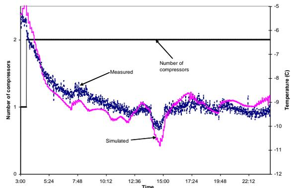
Figure 9: Closed system simulation with given schedule. Measured vs simulated brine temperature leaving chiller #1, and number of compressors in operation
