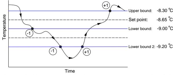
Figure 3: Variation of the brine temperature at the slab exit
