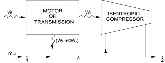
Figure 2: Model of the reciprocating compressor
