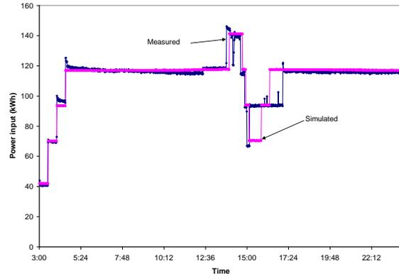
Figure 12: Closed system simulation with controller. Measured vs simulated total power input
