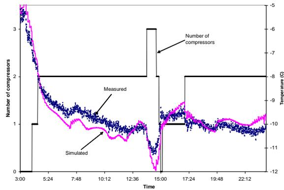
Figure 10: Closed system simulation with given schedule. Measured vs simulated brine temperatures leaving chiller #2, and number of compressors in operation
