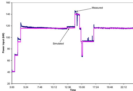
Figure 7: Open system simulation with given schedule. Measured vs simulated total power input
