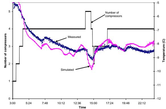
Figure 8: Closed system simulation with given schedule. Measured vs simulated brine temperature leaving the slab, and total number of compressors in operation
