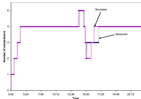
Figure 11: Closed system simulation with controller. Measured vs simulated number of compressors
