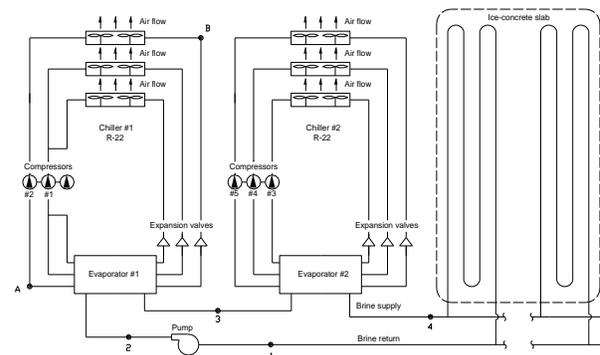
Figure 1: Schematic of the refrigeration system
