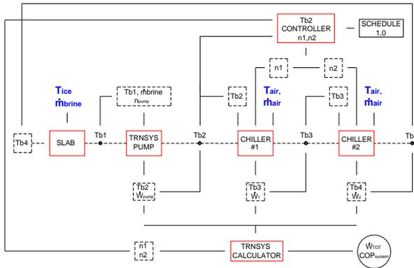
Figure 4: TRNSYS simulation flowchart
