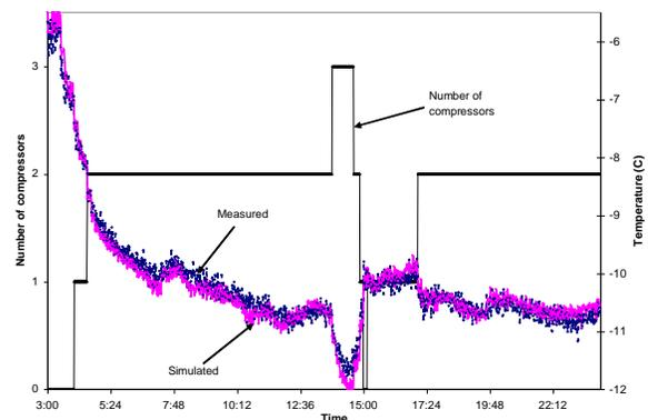
Figure 6: Open system simulation with given schedule. Measured vs simulated brine temperatures leaving chiller #2, and number of compressors in operation
