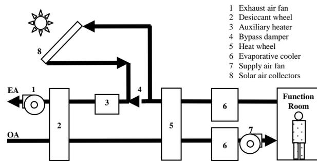
Fig. 1. Schematic diagram of solar desiccant cooling system.
