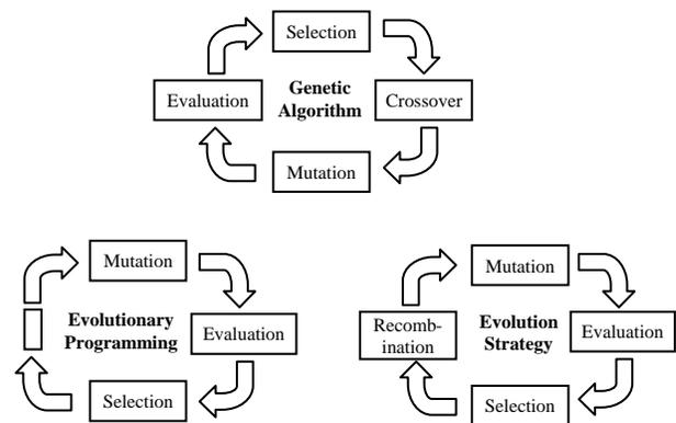
Fig. 2. Evolutionary loop of genetic algorithm, evolutionary programming and evolution strategy.
