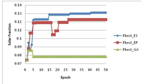
Fig. 3. Searching profile of best fitness (solar fraction) vs. epoch.
