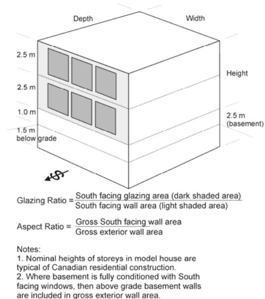
**Figure 2 – Example of base house model for generating parametric performance simulations.**
