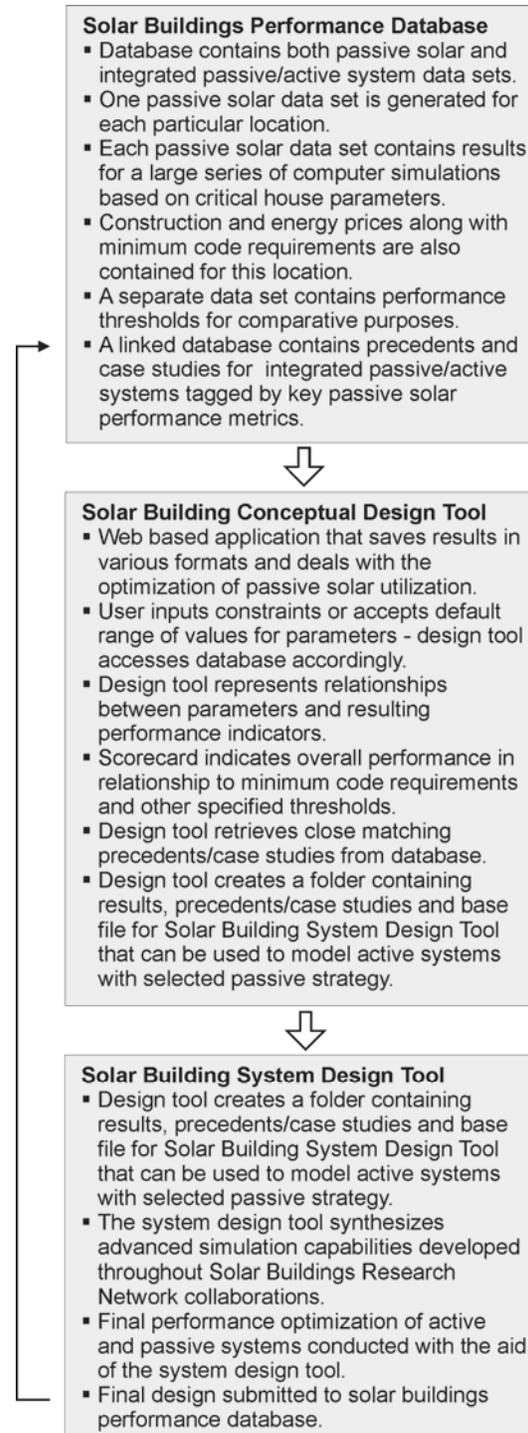
*Figure 1 – Proposed structure of data supporting solar building design tools.*
