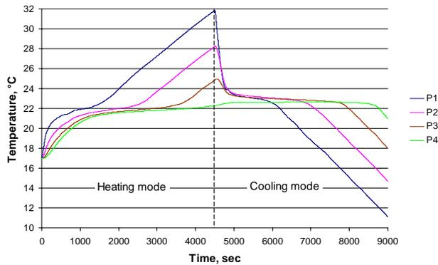
Figure 3 Temperature profile in the PCM for one heating and cooling cycle,  $T_{pc} = 22-23^{\circ}\text{C}$ , Case 1
