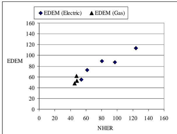
Figure 2: CO2 emissions (kg /m2 yr) – EDEM vs. NHER Surveyor.
