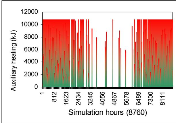
Figure 7: Auxiliary Heating Rate for TOU electric tank in Solar Model
