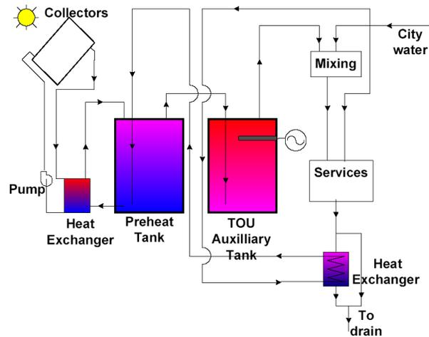
Figure 1: Schematic of Solar DHW Model
