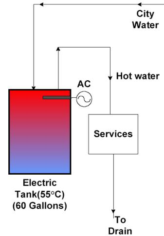
Figure 2: Schematic of Conventional Electric Tank Model
