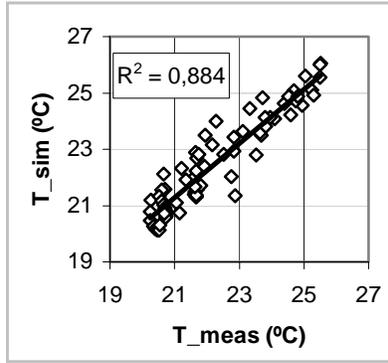
**FIGURE 2 – CORRELATION BETWEEN MEASURED AND SIMULATED INDOOR TEMPERATURES**
