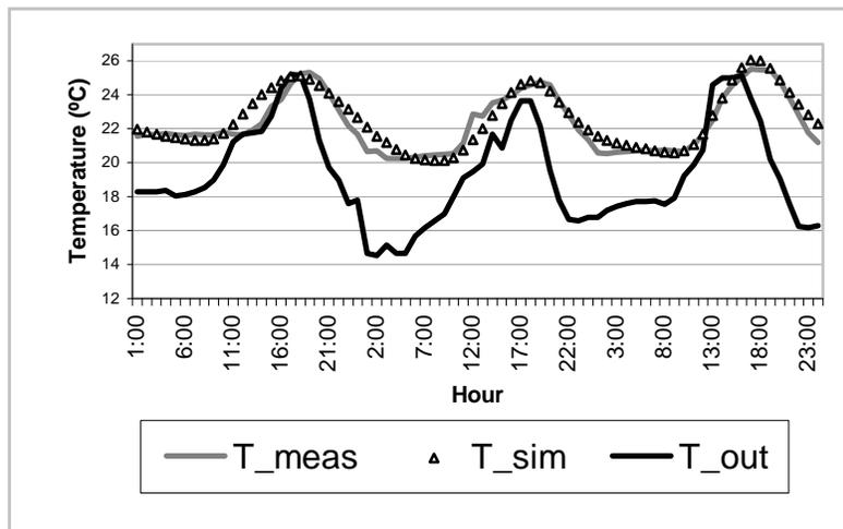
**FIGURE 3 – COMPARISON BETWEEN MEASURED AND SIMULATED INDOOR TEMPERATURES**
