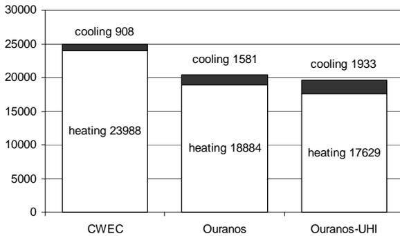
**Figure 6: Comparison of case house energy use (CWEC, Ouranos and Ouranos-UHI). Values are in kWh/year.**
