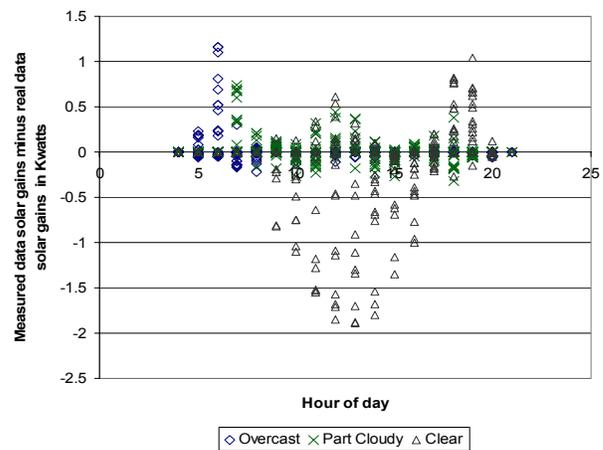
**Fig.2 Hourly difference between building solar gains using modelled and measured direct radiation, over July.**
