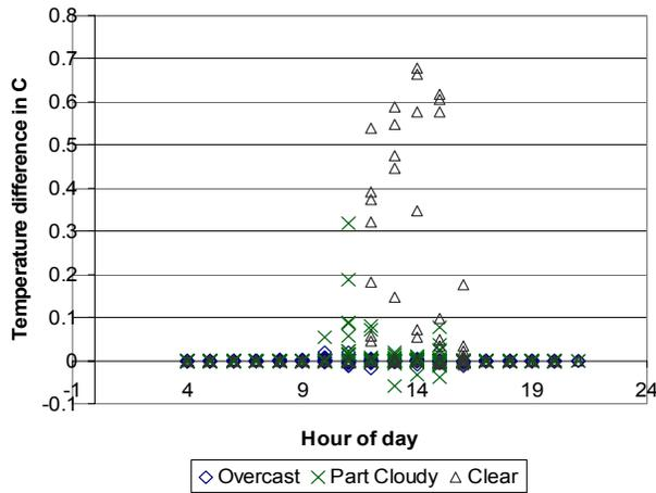
**Fig.3 Hourly difference in degrees C between building temperatures in winter using modelled and measured direct radiation.**
