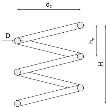
*Figure 3 – Coil dimensions.*
