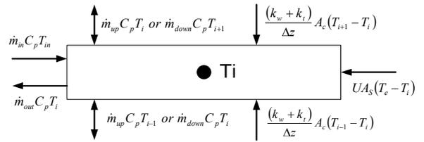
Figure 2 – Energy balance of tank node.
