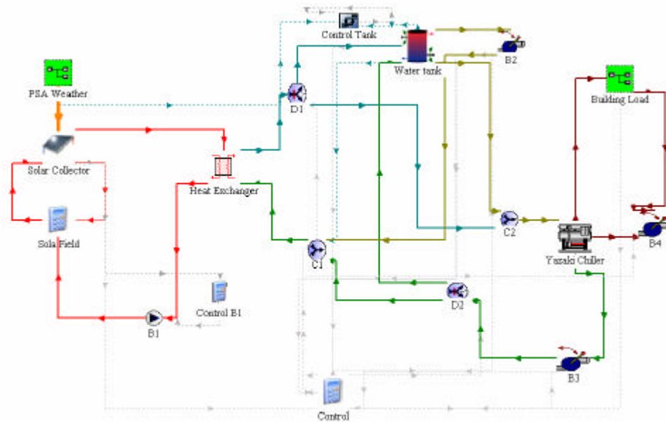
Figure 5: Configuration of the absorption system with external storage in TRNSYS
