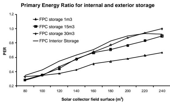
Figure 9: Primary energy ratio obtained for interior and exterior storage systems.
