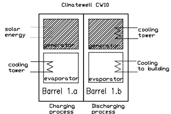
Figure 3: Components of the heat pump system with internal storage.
