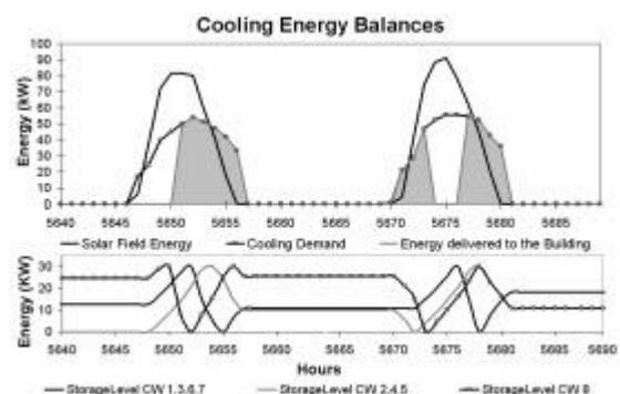
Figure 6: Energy balances of the solar cooling system with interior storage (Case 3).
