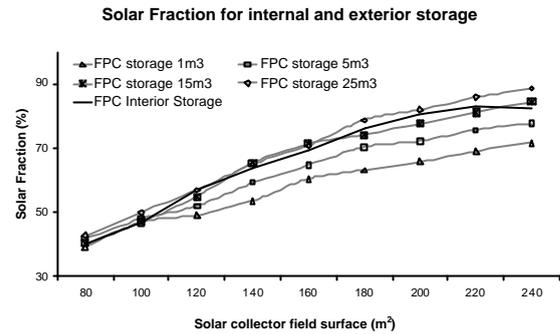
Figure 8: Solar fraction obtained for interior and exterior storage systems
