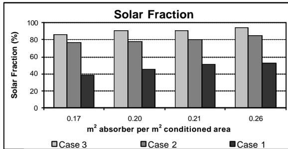
Figure 7: Cooling solar fractions. Comparison between the three cases modelled.
