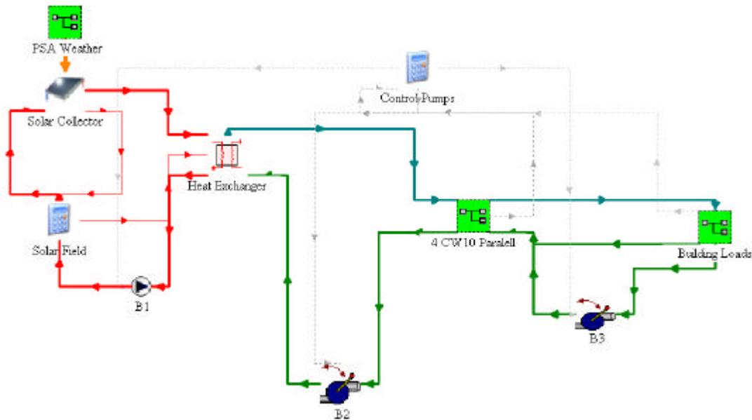
Figure 4: Configuration of the absorption system with internal storage in TRNSYS
