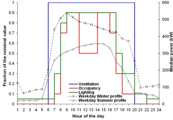
Figure 2 : Schedules used for weekdays and observed typical load profiles
