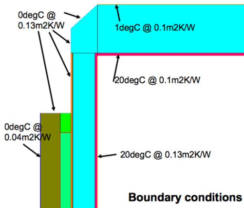
Figure 9: Materials & boundaries at a roof junction
