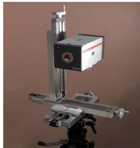
Figure 4: The camera holder equipped with micrometers in x, y and z direction.
