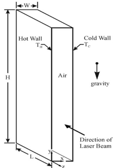
Figure 1: Experimental geometry and coordinate system.
