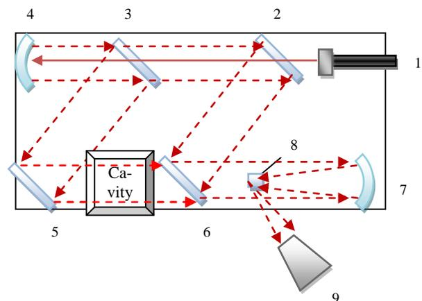
Figure 3: Plan view of a Mach-Zehnder interferometer
