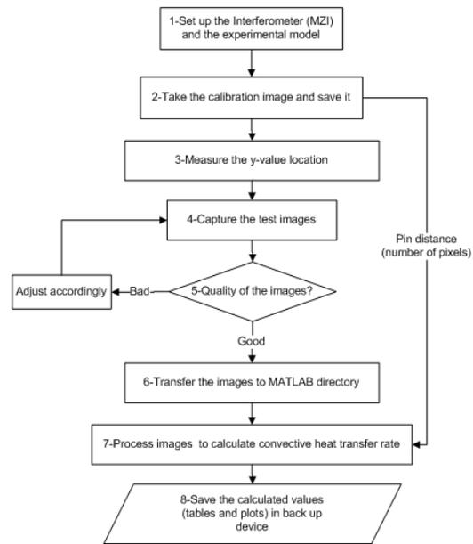
Figure 2: Steps in the current experiment to calculate Nusselt number
