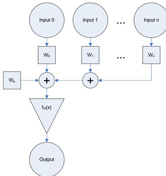
Figure 6: Basic processing elements of an ANN
