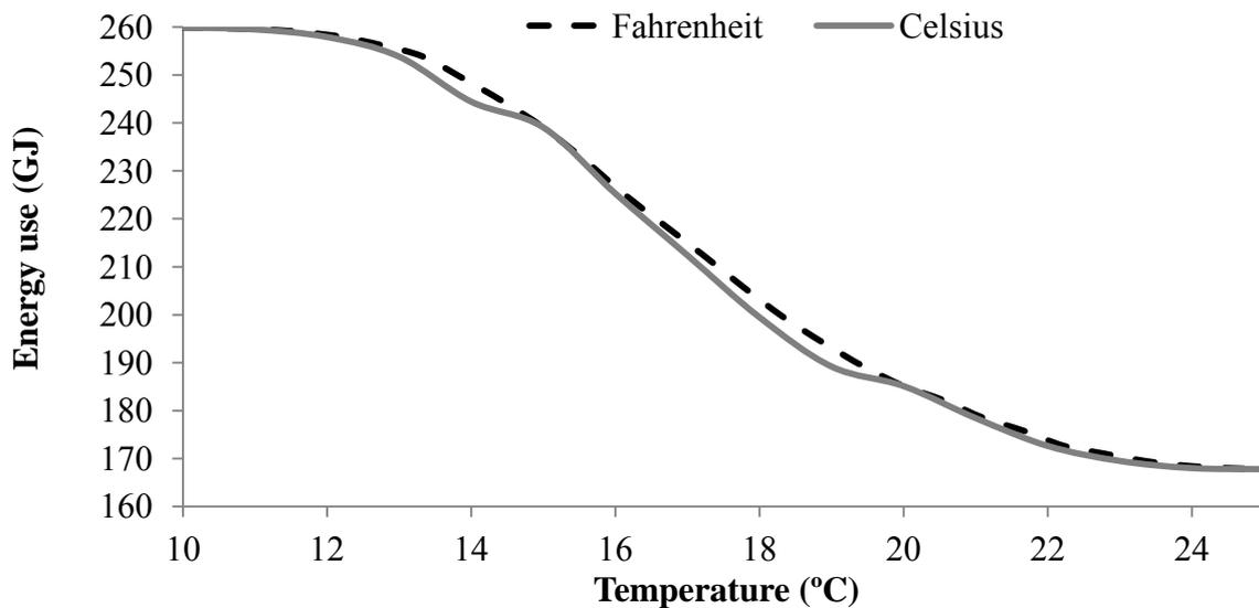
**Figure 3 - CDC System-2 Calgary modeled cooling energy use as a function of the air-side economizer shutoff temperature**
