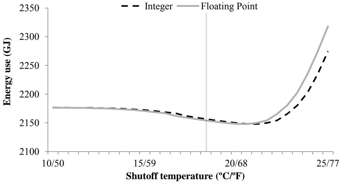
**Figure 6 - Cooling energy use versus economizer high limit shutoff temperature
