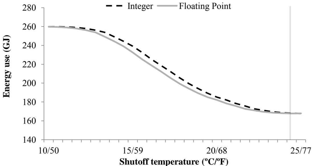
**Figure 7 - Cooling energy use versus economizer high limit shutoff temperature
