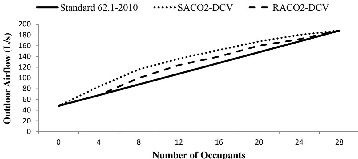
**Figure 4 – System outdoor airflow versus occupancy for both models compared to Standard 62.1-2010 minimum requirements**
