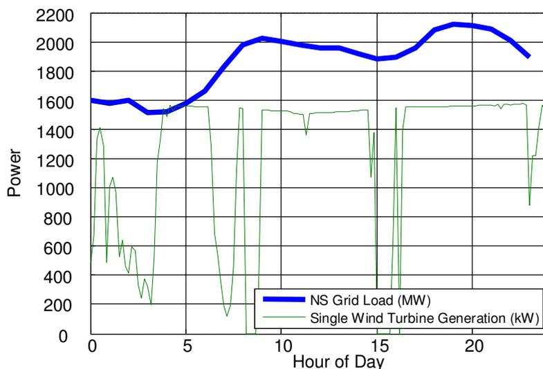
**Figure 1: Single Day Load Profile for the Nova Scotia Electricity Grid Feb 2, 2010 with 1.5 MW Wind Turbine Output Based on (Nova Scotia Power Inc. 2011)**
