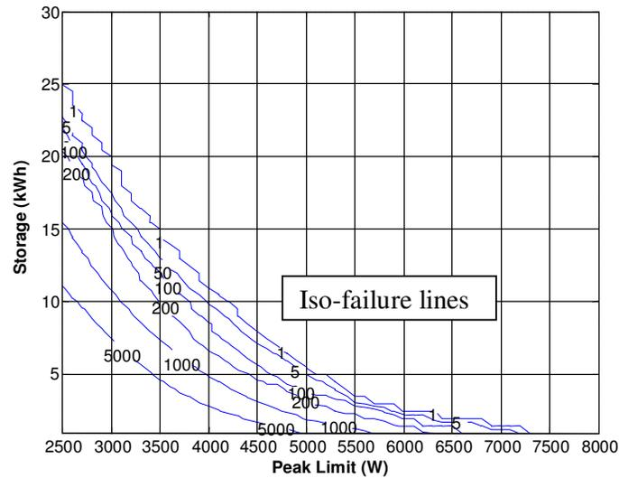
**Figure 5: 2D Iso-Failure Plot of energy storage (AT Region, Storage vs. Peak Limit)**
