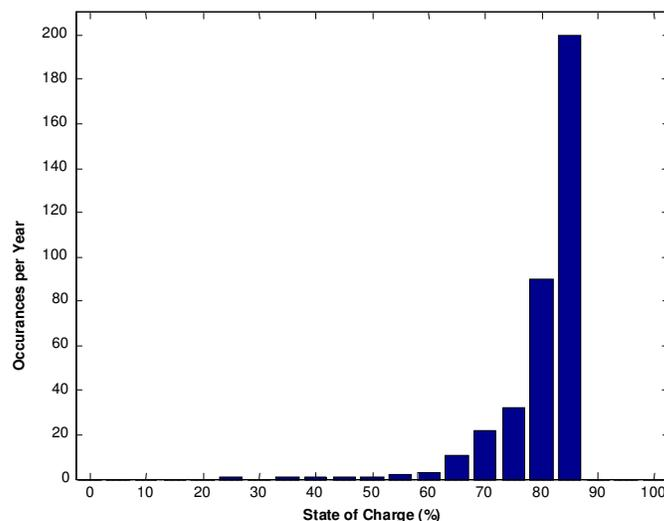
**Figure 8: Histogram of Lowest Battery State of Charge Experienced Each Day of a Year (AT Region)**
