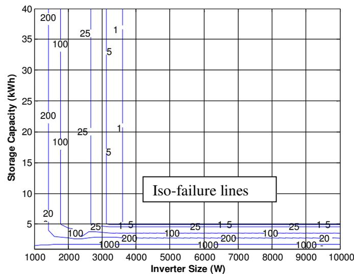
**Figure 7: 2D Iso-Failure Plot (AT Region, 5260 W Peak Limit, Storage vs. Inverter Size)**
