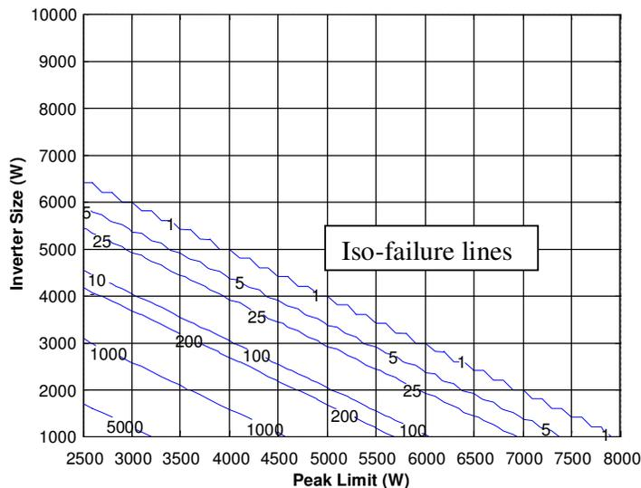
**Figure 6: 2D Iso-Failure Plot of power (AT Region, Inverter Size vs. Peak Limit)**
