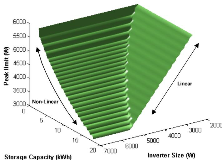
**Figure 4: 3D Iso-Failure Surface Plot of energy storage and power (AT Region, 1 Failure Event Surface)**
