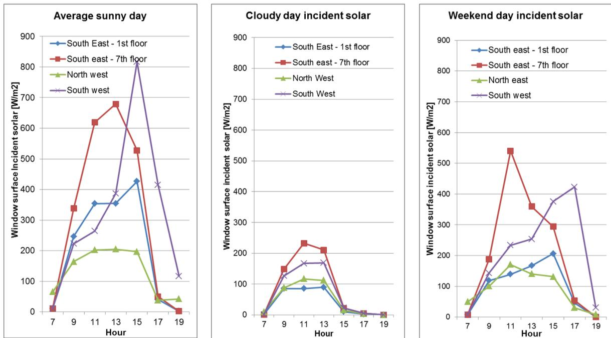
**Figure 7: The incident light conditions were estimated using EnergyPlus and SIMEB weather data for Ottawa. Due to the neighbouring building, the incident solar radiation is different on the 1<sup>st</sup> and 7<sup>th</sup> floor on the SE facade.**
