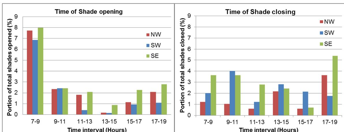
**Figure 8: Time when shades are opened (left) and closed (right), expressed as a fraction of the total number of shades.**
