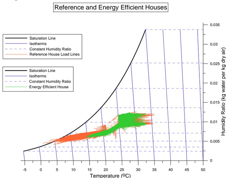
**Figure 4: Load lines for reference and energy efficient houses overlaid on each other**
