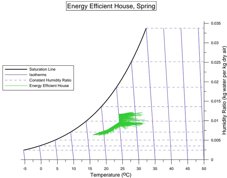
**Figure 6: Load lines plotted for the energy efficient house in spring (20 March to 20 June)**
