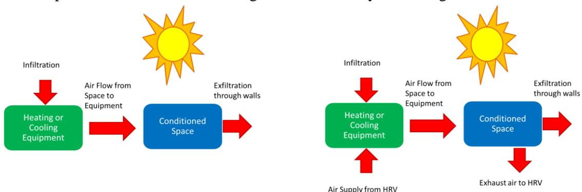
**Figure 1: Diagrams showing the air flows for the reference house and the energy efficient house with HRV**
