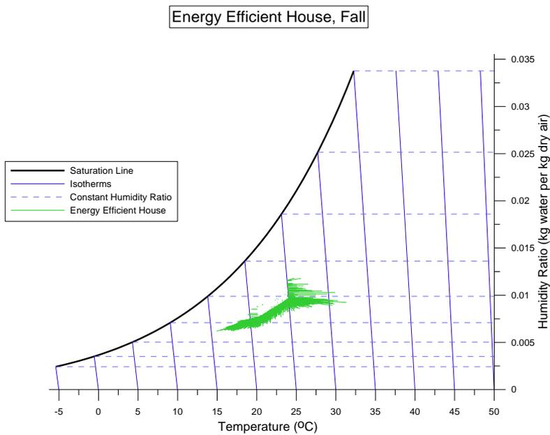
**Figure 10: Load lines plotted for the energy efficient house in fall (22 September to 20 December)**
