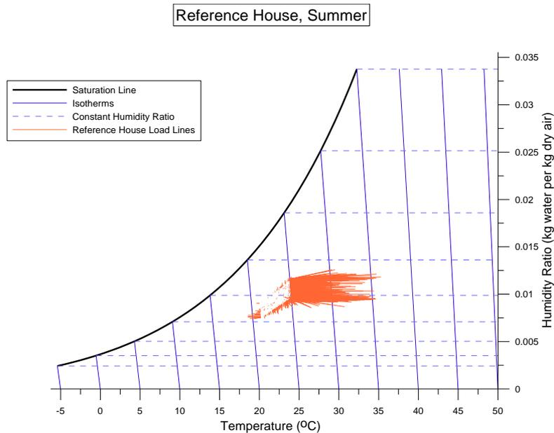
**Figure 7: Load lines plotted for the reference house in summer (21 June to 21 September)**
