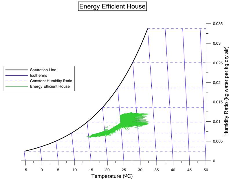
**Figure 3: Load lines for energy efficient house plotted on psychrometric chart**
