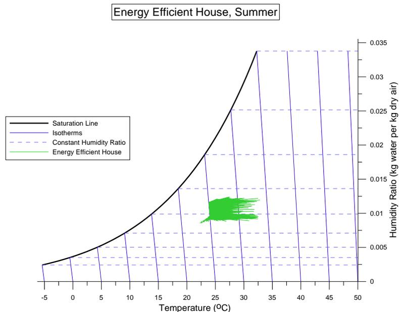
**Figure 8: Load lines plotted for the energy efficient house in summer (21 June to 21 September)**
