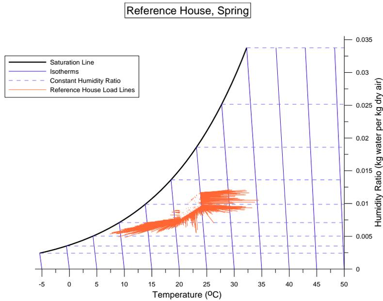
**Figure 5: Load lines plotted for the reference house in spring (20 March to 20 June)**
