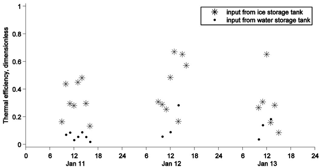
Figure 6: Thermal efficiency of solar thermal collectors from Jan. 11 to Jan. 13
