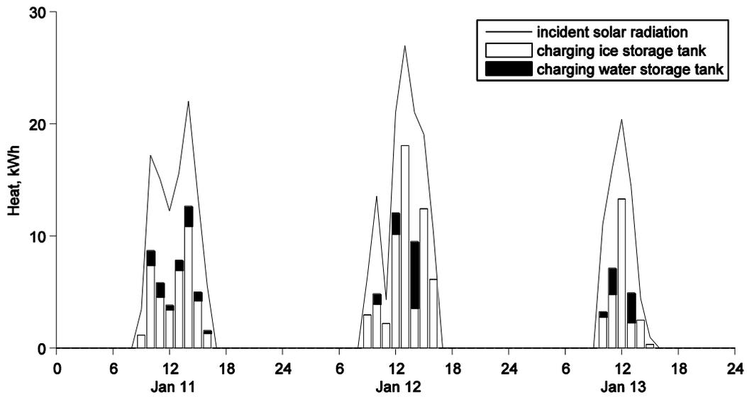
Figure 5: Solar incidence and storage of solar combisystem from Jan. 11 to Jan. 13
