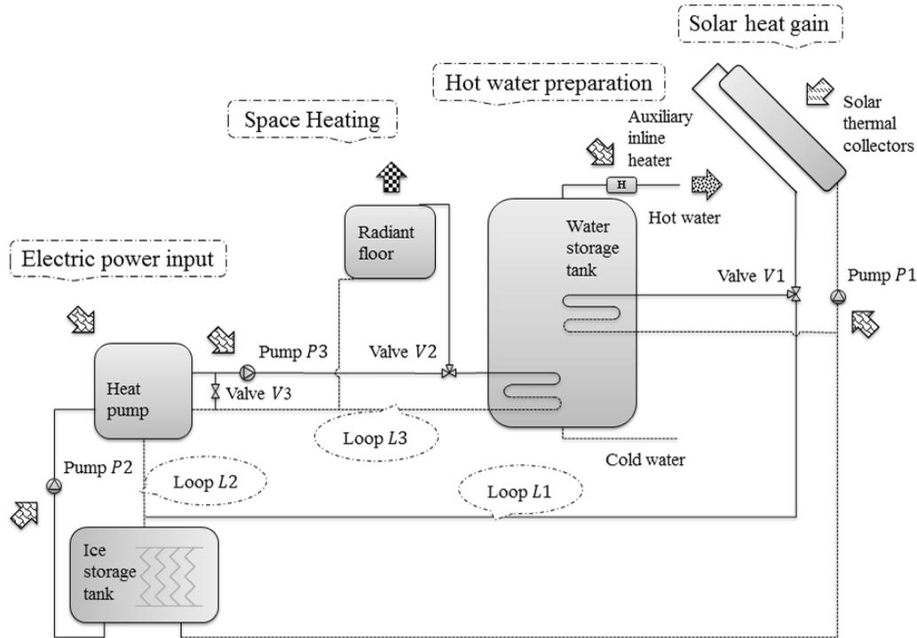
**Figure 1: Schematic of solar combisystem configuration**
