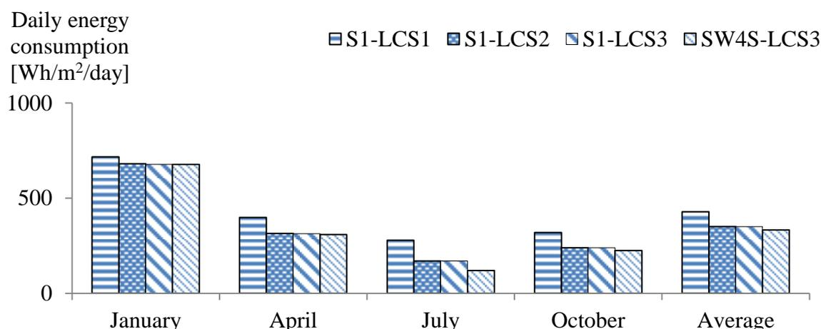
**Figure 6: Effect of smart window opacity state control with lighting control LCS3 on building energy consumption compared to passive states**
