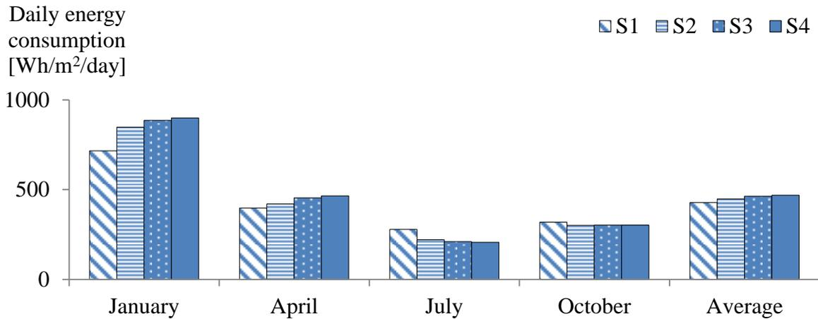
**Figure 3: Effect of window passive opacity state on building loads with light control LCS1**
