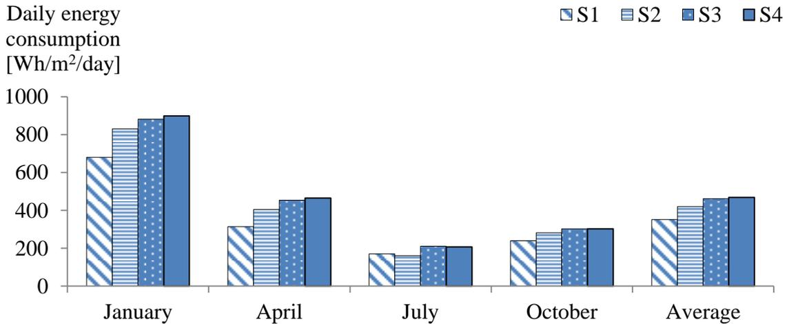
**Figure 4: Effect of window passive opacity state on building loads with light control LCS2**
