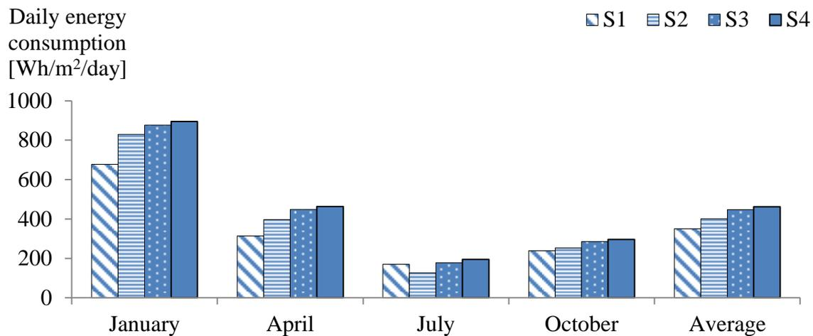
**Figure 5: Effect of window passive opacity state on building loads with light control LCS3**
