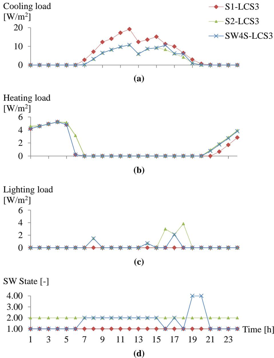
**Figure 7: Hourly results for a typical day of July – a) Cooling loads, b) Heating loads, c) lighting loads and d) Smart window optimized opacity state**
