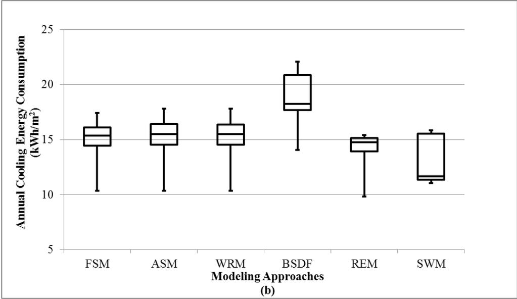
**Figure 2: (b) Boxplot of the cooling energy consumption showing the maximum, upper quartile, median, lower quartile and the minimum values for the six modelling approaches.**
