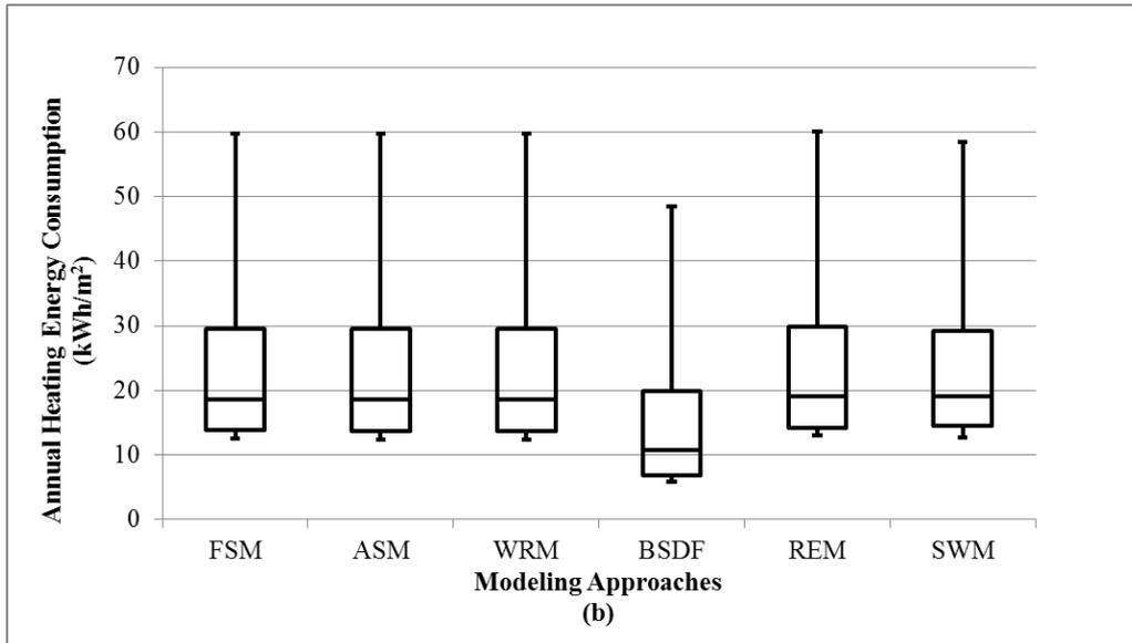
**Figure 1: (b) Boxplot of the heating energy consumption showing the maximum, upper quartile, median, lower quartile and the minimum values for the six modelling approaches.**
