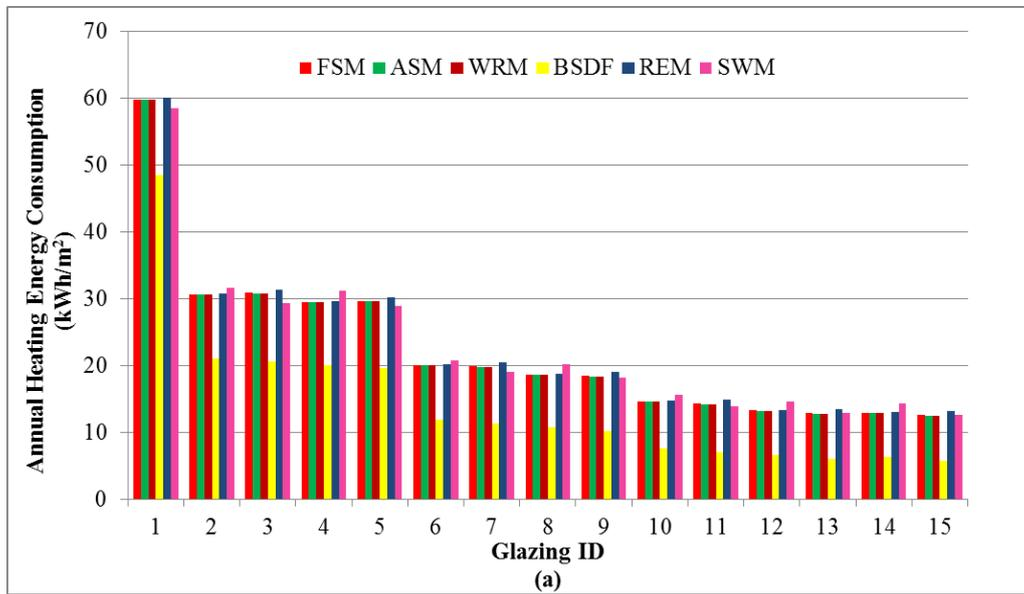
**Figure 1: (a) Heating energy consumption predicted by six modelling approaches**
