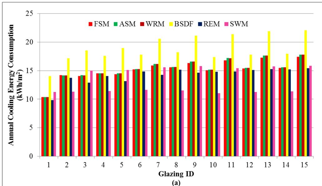
**Figure 2: (a) Cooling energy consumption predicted by six modelling approaches**
