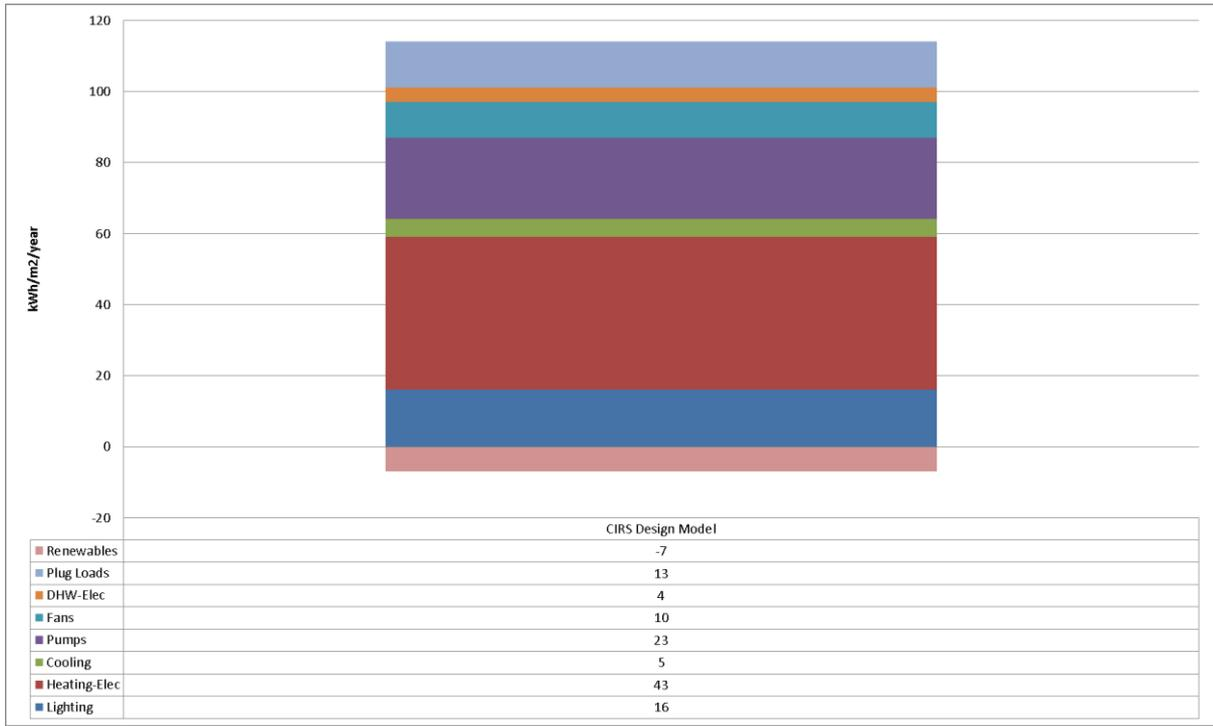
**Figure 1: Annual Energy Utilization Intensity by End Use (kWh/m2/year) (Stantec Cons., 2010)**
