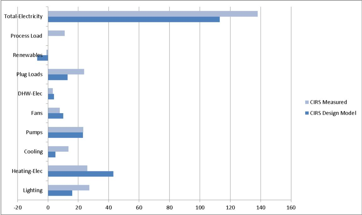
**Figure 5: Comparison of Measured Data with Design Model by CIRS Annual Energy Utilization Intensity by End-Use (kWh/m2/year)**
