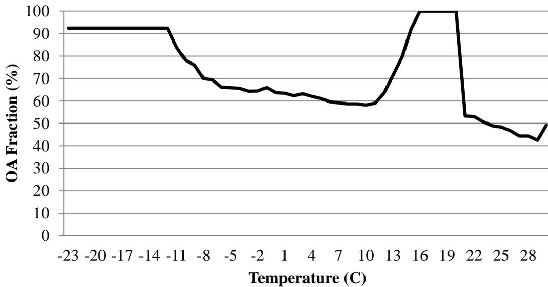
**Figure 10 –AHU2 OA fraction relative to OAT from DOE2 code generated by EE4 interface.**
