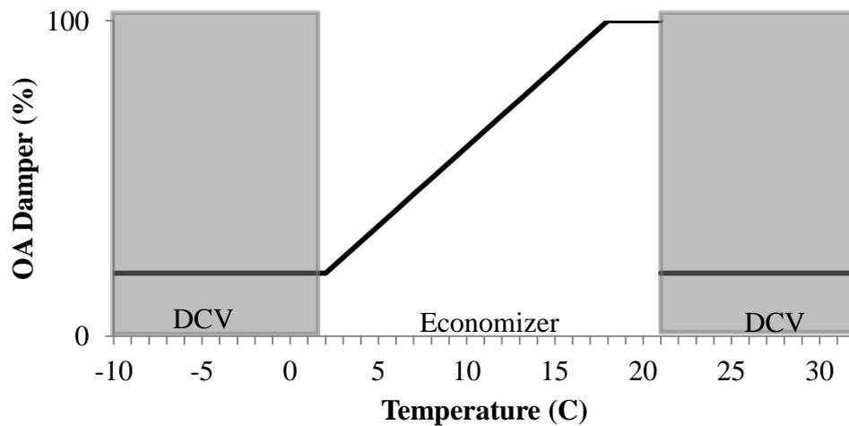
**Figure 3 - CDC EE4-DOE2 model air-side economizer and DCV control regions**
