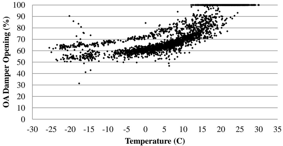
**Figure 7 - 2011 AHU2 OA damper opening relative to OAT**
