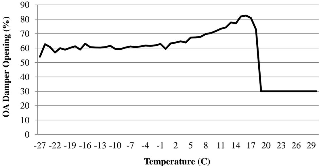
**Figure 6 - 2010 average AHU2 OA damper opening at each OAT**
