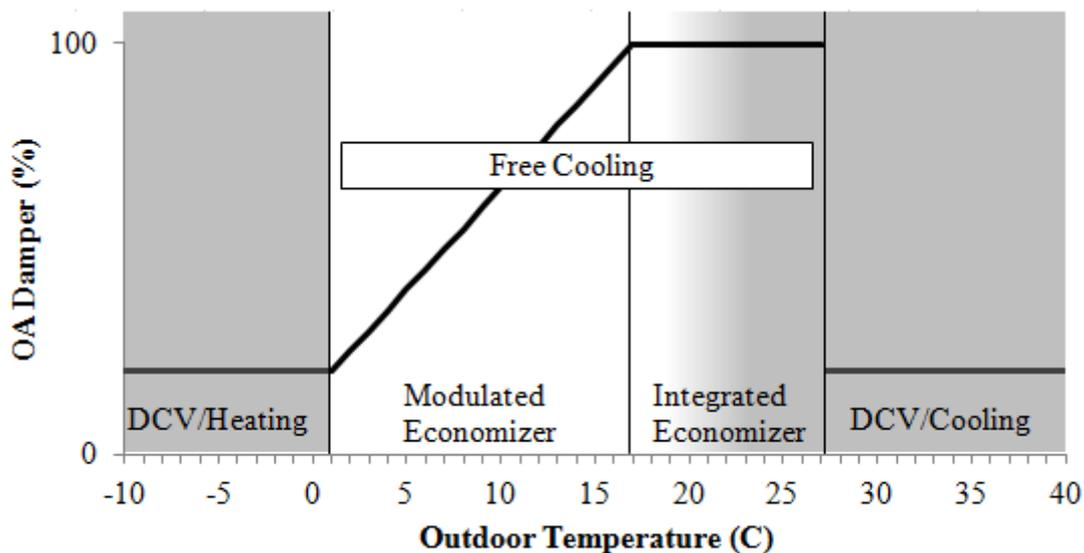
**Figure 1 – Theoretical economizer and DCV operation**
