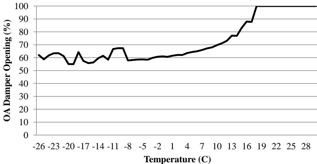
**Figure 8 - 2011 average AHU2 OA damper opening at each OAT**
