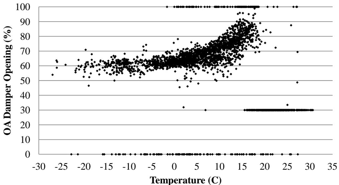
**Figure 5 - 2010 AHU2 actual OA damper opening relative to OAT**
