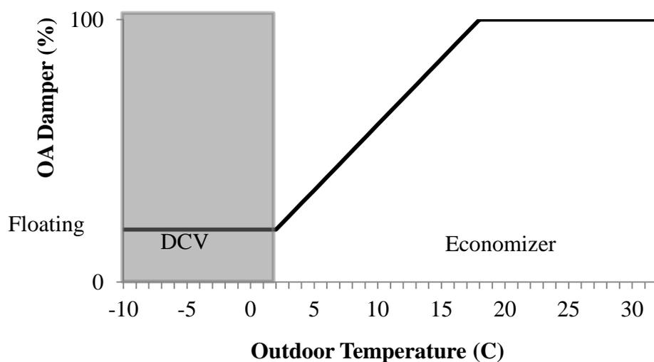
Figure 2 – AHU2 air-side economizer and DCV operation
