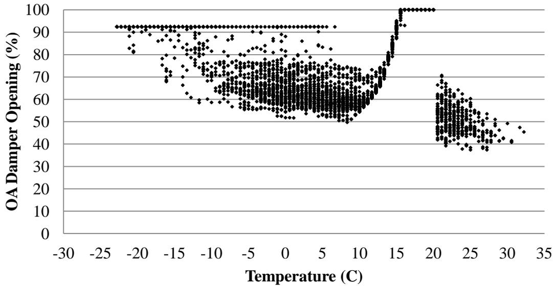
**Figure 9 –AHU2 OA damper opening relative to OAT from DOE2 code generated by EE4 interface.**
