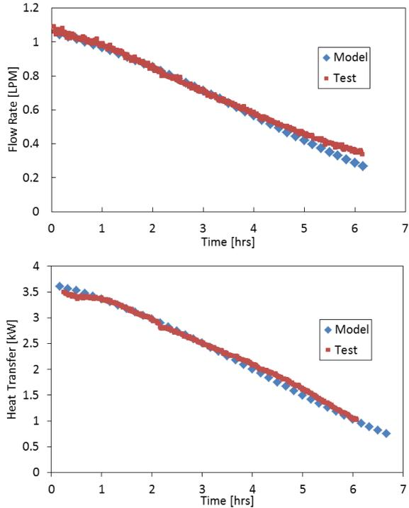
**Fig. 10: Thermosiphon flowrate and heat transfer (Test 1).**
