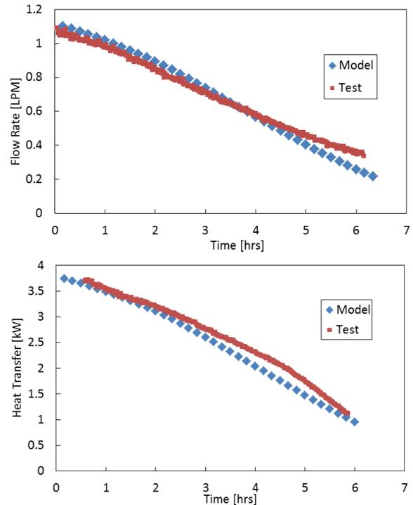
**Fig. 11: Thermosiphon flowrate and heat transfer (Test 2).**
