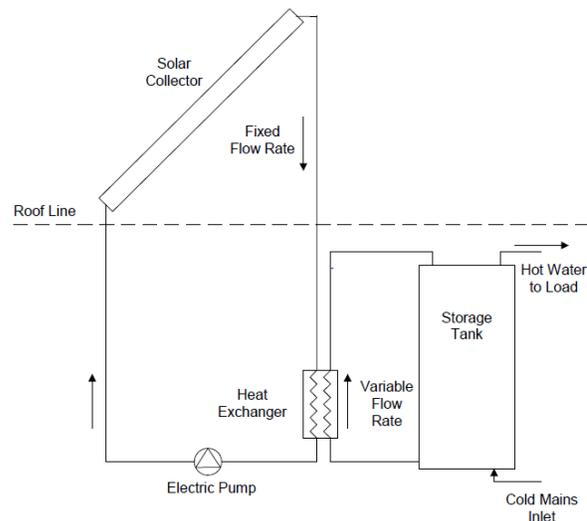
**Fig. 1: Schematic of simple SDHW system with external heat exchanger.**
