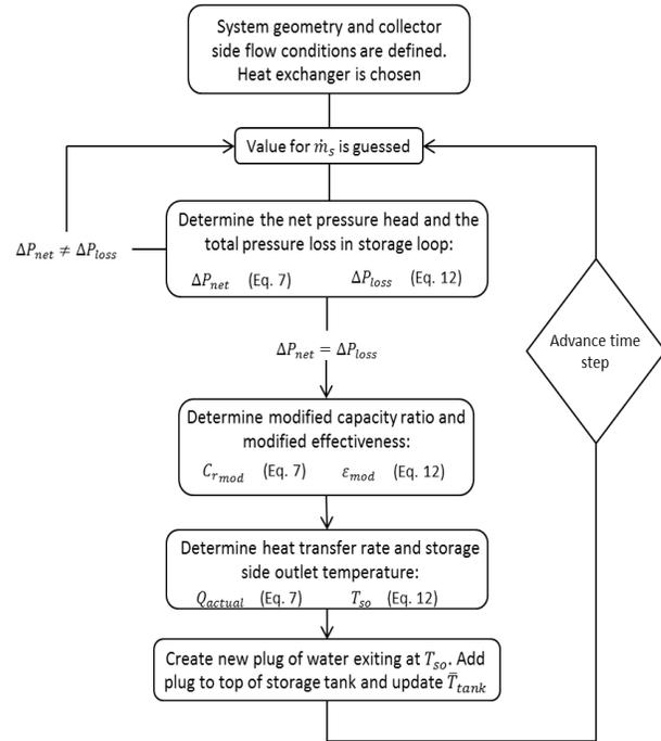
**Fig. 6: Flow chart outlining model's iterative method.**
