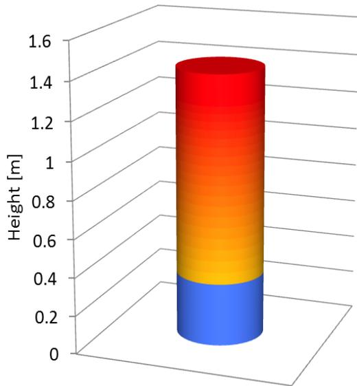
Fig. 7: Calculated storage tank temperature profile.
