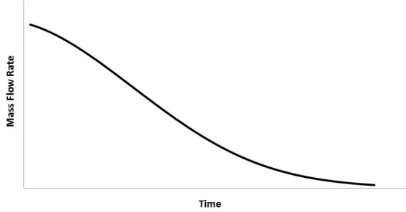
**Fig. 4: Flow profile of a thermosiphon during storage tank charging.**
