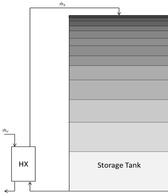
**Fig. 5: Stratification profile within a storage tank.**
