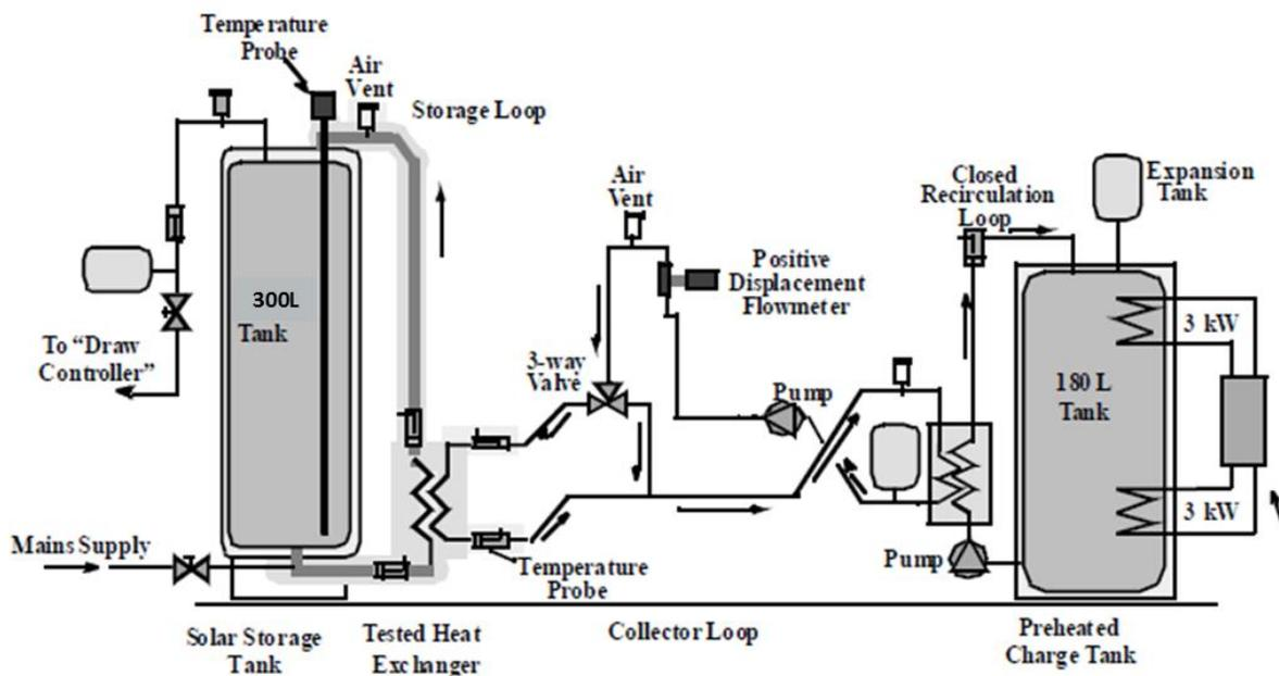
Fig. 8: Schematic of testing apparatus used in full-scale experiment
