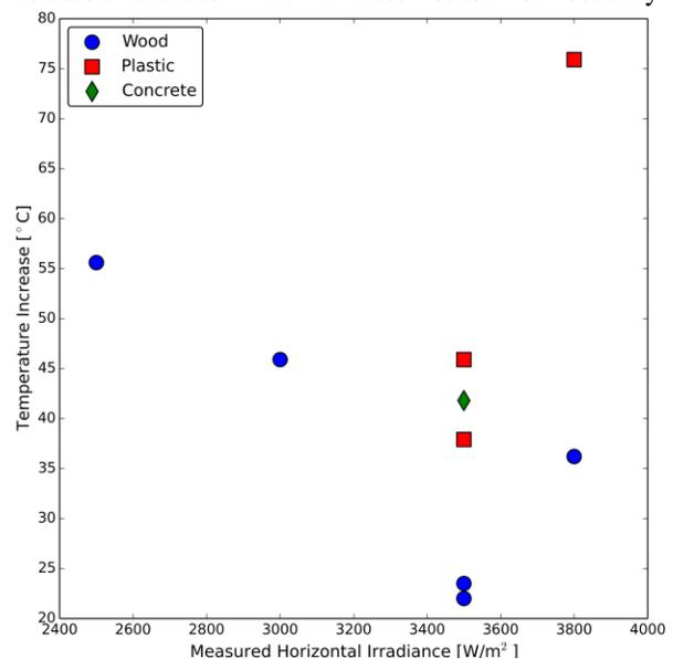
**Figure 2.** Measured temperature gains vs. reflection intensity.
