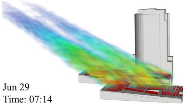
**Figure 3.** Point-in-time rendering of reflection impact from a PV array
