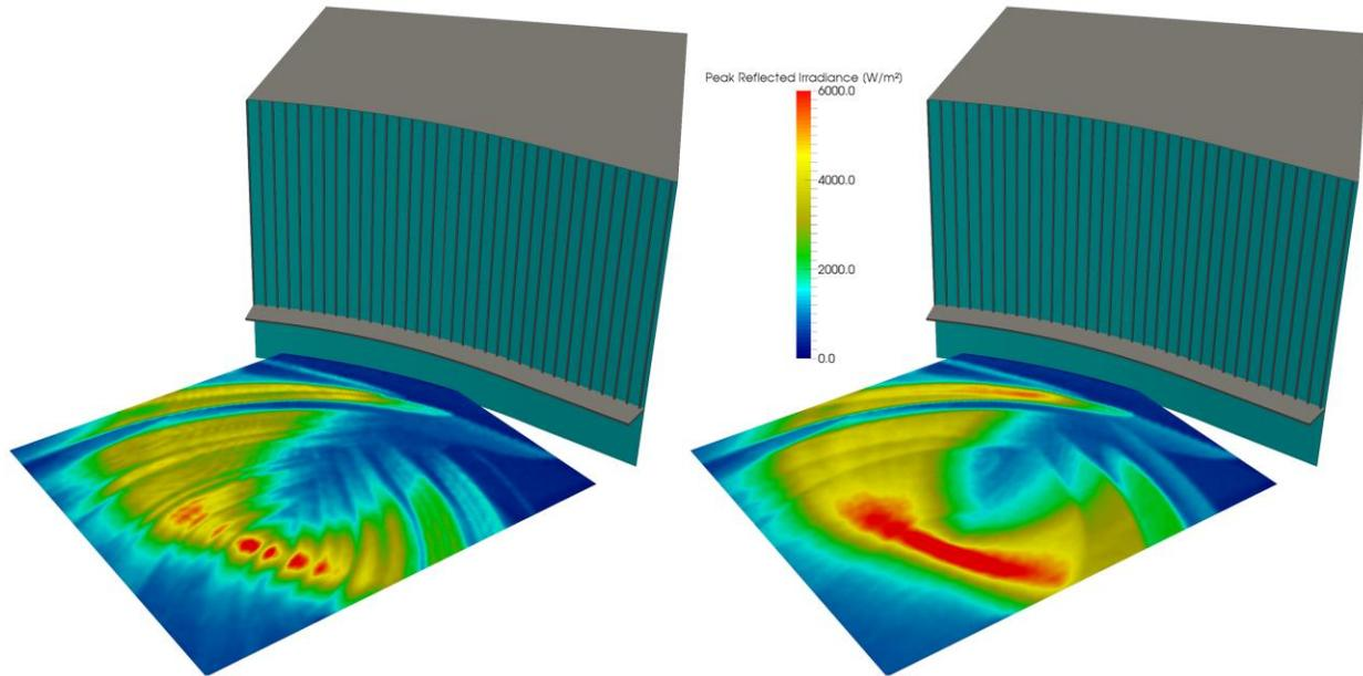
**Figure 1.** Comparison of predicted hourly peak reflected irradiance for 'typical' (left) and 'clear sky' (right) ambient solar conditions.
