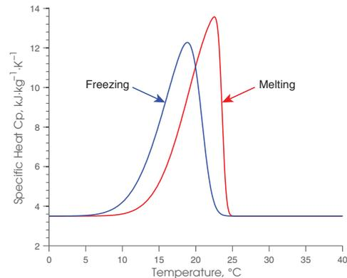
Figure 4: Specific heat as a function of PCM temperature. In this study, only the freezing curve is considered.
