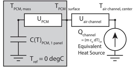
Figure 1: (Left) simplified first-order model and (right) PCM-TES model. During the training stage, the heating/cooling, internal gains and solar gains in the simplified office come from the EnergyPlus simulation results. During the analysis stage, the heating/cooling supplements the heat discharged from the PCM-TES.
