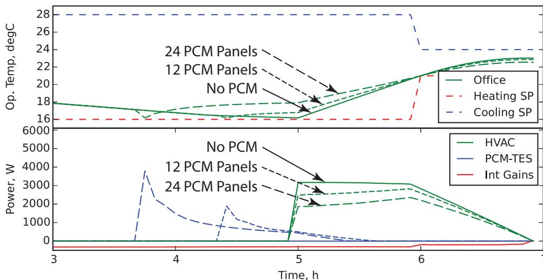
Figure 6: Office temperature, HVAC and PCM-TES supplied heat depending on three cases: (1 – solid line) when no PCM is used, (2 – short dash) a PCM-TES with 12 panels is used and (3 – long dash) a PCM-TES with 24 panels is used. The HVAC is allowed to be used starting at 5:00 AM.
