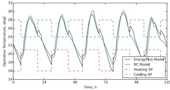
Figure 2: EnergyPlus and first-order model room temperatures.
