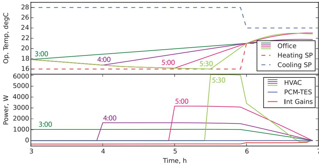
Figure 5: Office temperature and HVAC supplied heat depending on the time when HVAC is allowed to be used.
