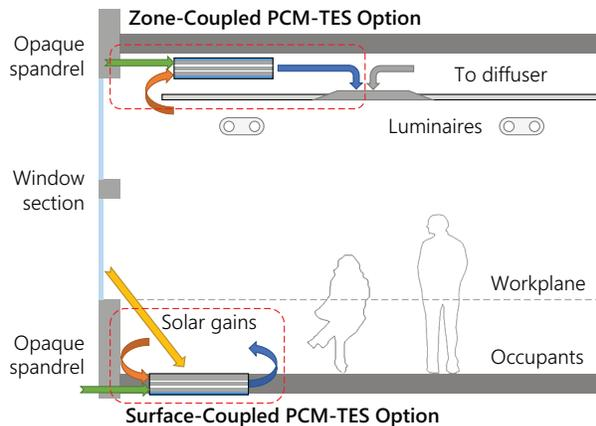
Figure 3: PCM-TES configurations: zone-coupled and surface-coupled.
