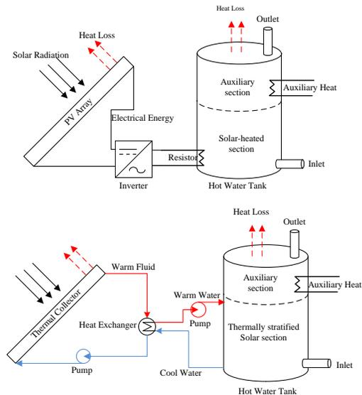
Fig 1. Simplified layout of the DHW systems. (a) PV configuration, (b) solar thermal configuration
