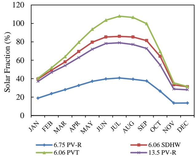
Fig 2. Simulated monthly solar fraction for Toronto
