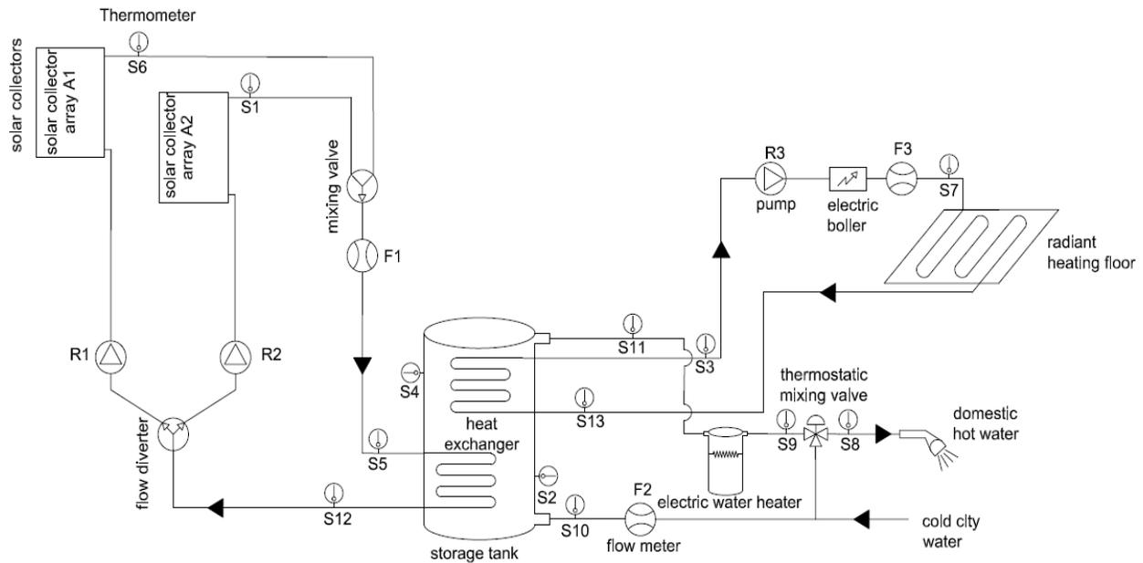
Figure 1. Scheme of the monitored solar thermal combisystem
