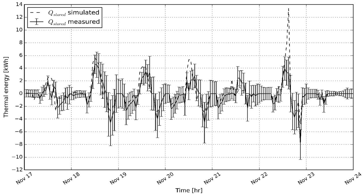
Figure 4. Comparison of the measured and simulated thermal energy stored in the storage tank from November 17 to November 23, 2014
