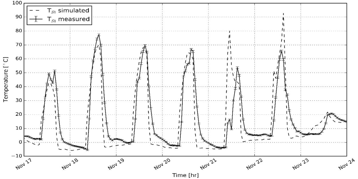
(b) Heat-transfer fluid temperature  $T_{S1}$  of the array A2
