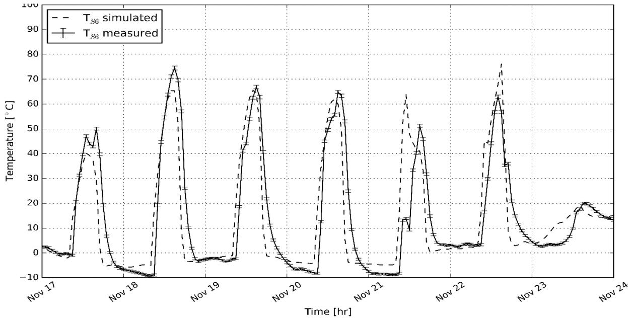
(a) Heat-transfer fluid temperature  $T_{S6}$  of the array A1
