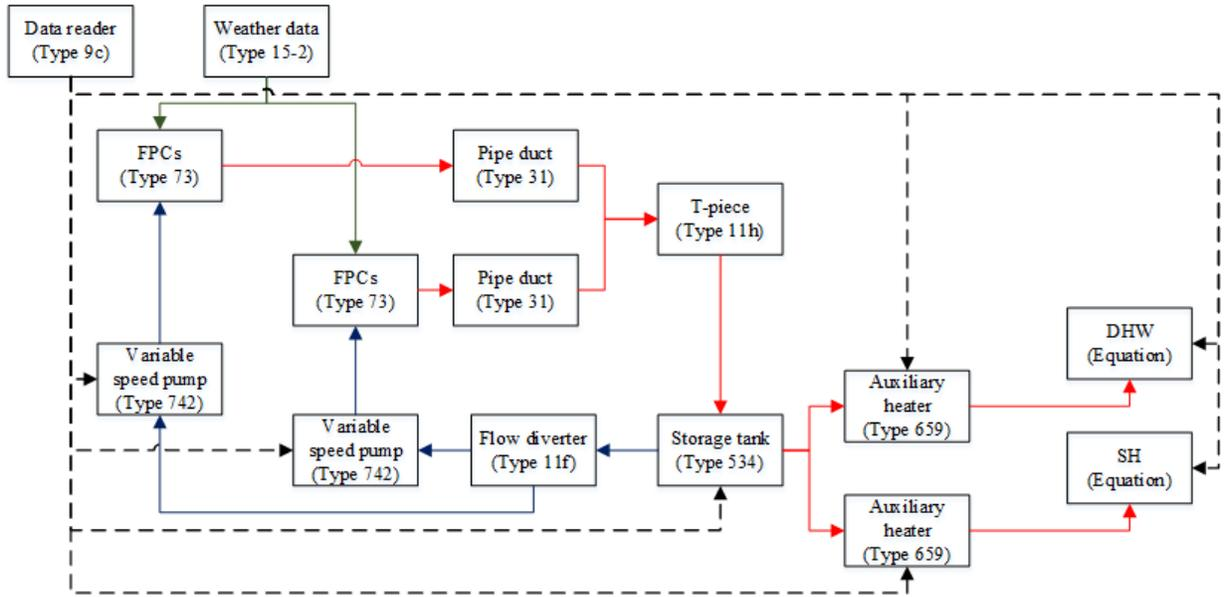
Figure 2. Flow diagram for the TRNSYS solar combisystem model
