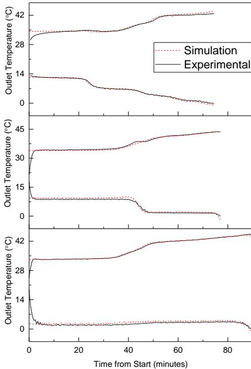
Figure 3: Comparison of simulated and experimental heat pump source and load outlet temperatures under 3 different source and load flow rates with water as the source fluid
