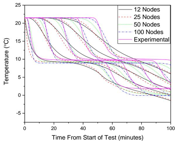
Figure 13: Node sensitivity analysis using a cold thermal storage tank with a 50/50 water/glycol solution as the storage medium
