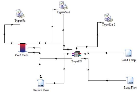
Figure 5: TRNSYS model containing data readers for the load conditions and source flow rate for tank Type 534
