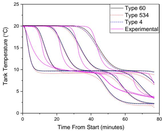
Figure 14: Comparison of TRNSYS Type 60, 534 and 4 when modelling a cold thermal storage tank using water as the storage medium
