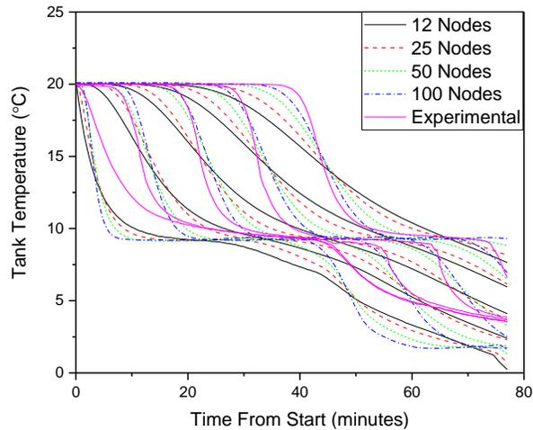
Figure 12: Node sensitivity analysis using a cold thermal storage tank with water as the storage medium
