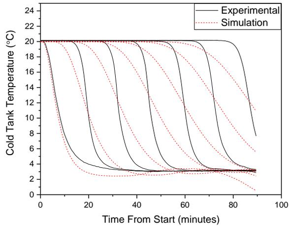
Figure 6: Tank temperature profile at a source flow rate of 3 L/min and a load flow rate of 3 L/min
