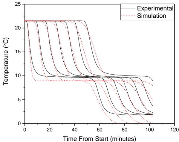
Figure 10: Tank temperature profile at a source flow rate of 5 L/min and a load flow rate of 3.5 L/min
