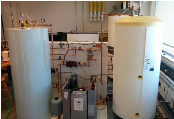
*Figure 2: Experimental set-up with the cold thermal storage on the left and hot thermal storage on the right (before insulating pipes)*
