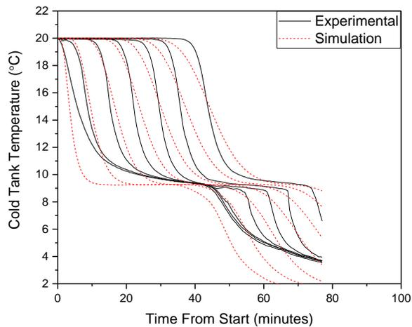
Figure 7: Tank temperature profile at a source flow rate of 6 L/min and a load flow rate of 6 L/min
