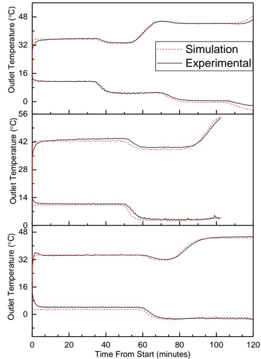
Figure 4: Comparison of simulated and experimental heat pump source and load outlet temperatures under 3 different source and load flow rates with a glycol solution as the source fluid
