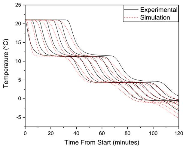
Figure 11: Tank temperature profile at a source flow rate of 7.5 L/min and a load flow rate of 5.5 L/min
