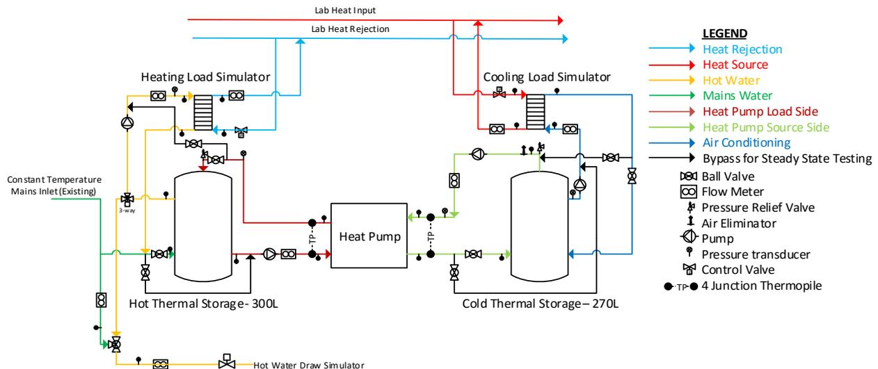
Figure 1: Schematic of experimental test set-up
