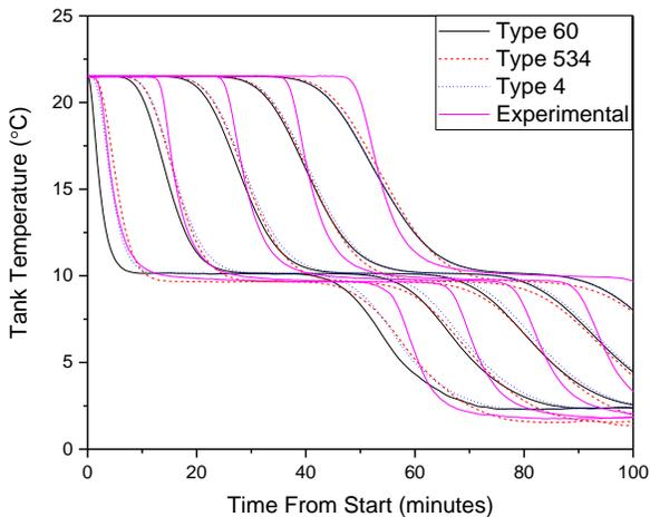
Figure 15: Comparison of TRNSYS Type 60, 534 and 4 when modelling a cold thermal storage tank using a water/glycol solution as the storage medium
