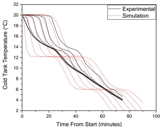
Figure 8: Tank temperature profile at a source flow rate of 9 L/min and a load flow rate of 6 L/min
