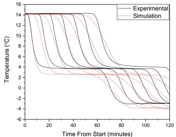
Figure 9: Tank temperature profile at a source flow rate of 4 L/min and a load flow rate of 4 L/min
