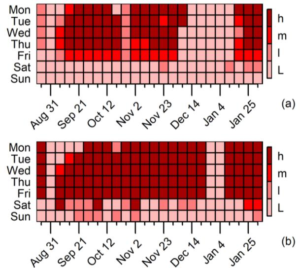
Figure 8: Occupancy profiles (a) measured retroactively with Wi-Fi and (b) forecasted during the implementation period with electrical load.
