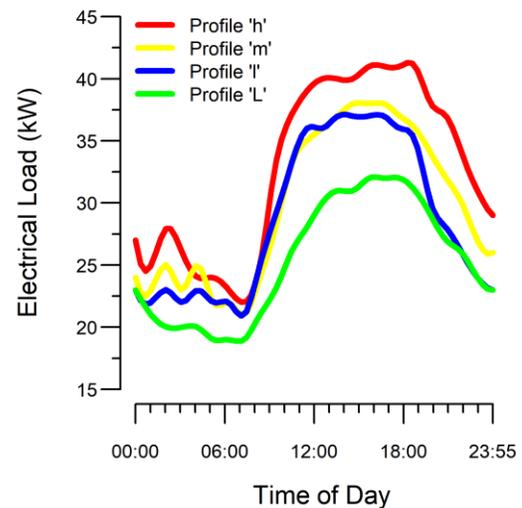
Figure 4: Representative plug-in equipment and lighting load profiles previously developed for the building.
