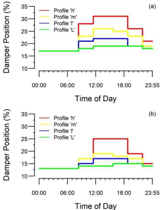
Figure 3: Damper position profiles for (a) AHU1 and (b) AHU2
