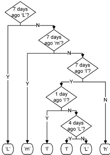
Figure 5: Classification tree for day-ahead occupancy prediction using previous week of electrical load profiles.
