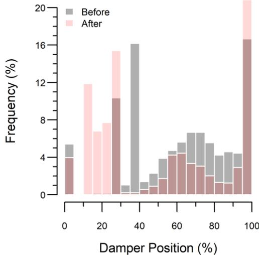
Figure 7: Outdoor air damper positions from the baseline (before) and implementation (after) period.
