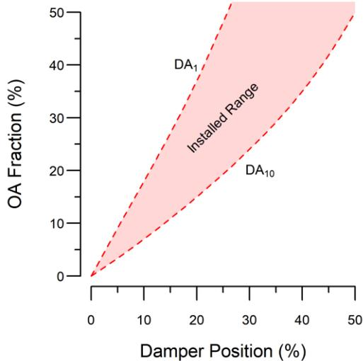
Figure 2: Damper position and air fraction for opposed blade dampers.
