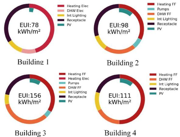
Figure 6: EUI Values based on Digital Twin Model
