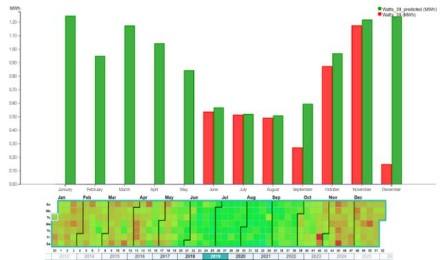
Figure 5 – Data Generation using Machine Learning integrated within IES-iSCAN and incorporating data from Physics Based IES-VE model for Building 4.
