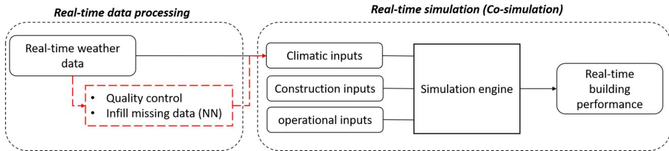
Figure 3- Placement of method of this study (red dashed line) in a real-time building simulation.
