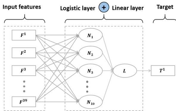
Figure 2 - Diagram of the vanilla neural network utilized in this study.
