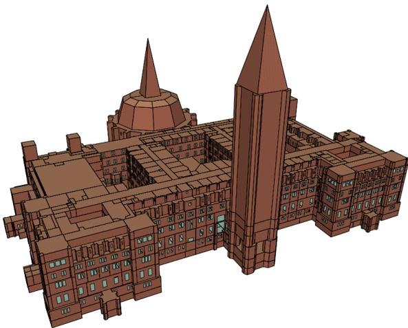
Figure 1: The geometry of the IES VE energy model of the existing Centre Block.
