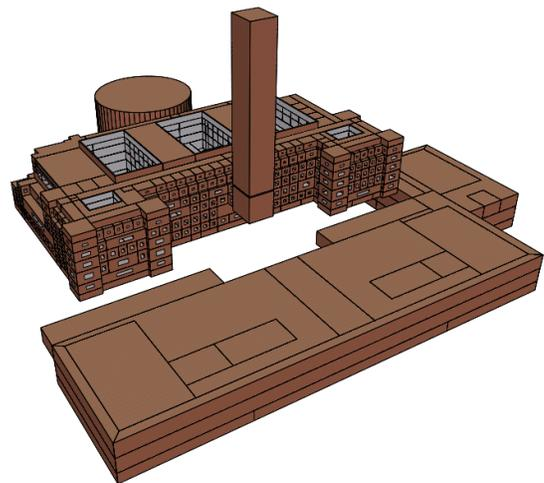
Figure 3: Geometry of the IES VE energy model used in the CBR Net-Zero Carbon Feasibility Study. Includes the CB potential skylights over courtyards and a core-and-shell representation of the potential PWC design.
