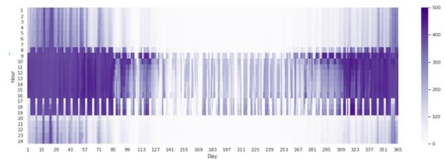
Figure 4: A heat map of useful heat recovered from the HRL (kW).
