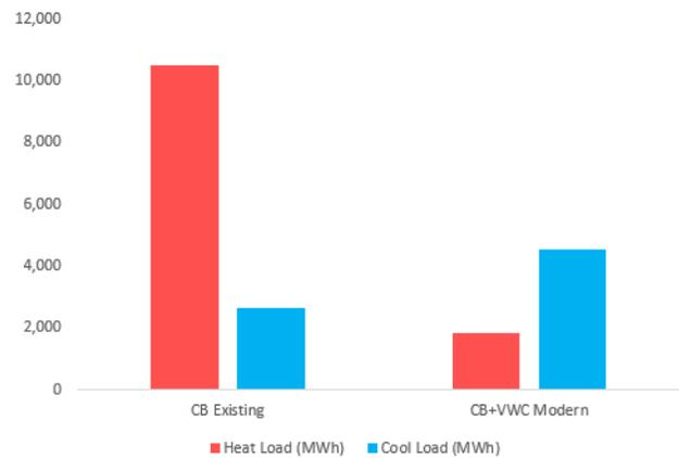
Figure 2: Annual heat and cool loads (MWh) from the IES VE energy model of existing CB compared to the baseline design (Option A) of the CBR Net-Zero Carbon Feasibility Study
