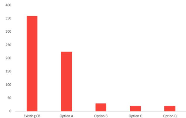
Figure 5: GHG intensity of delivered heat (g eCO<sub>2</sub> / kWh) of the existing Centre Block and four design options produced in the CBR Net-Zero Carbon Feasibility Study.
