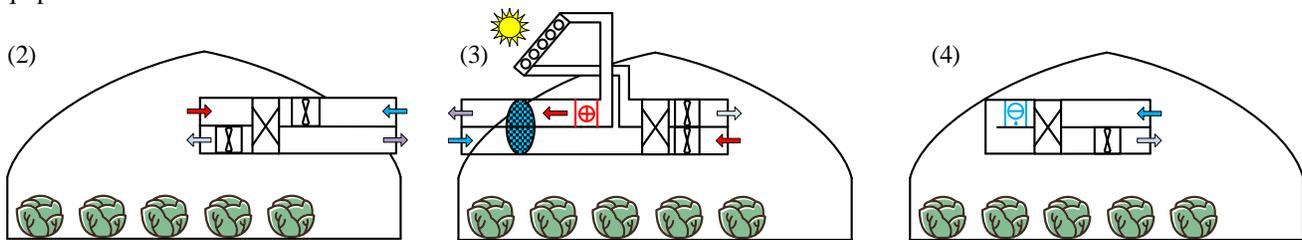
Figure 5 : Systems installed to assess the proposed humidity control strategies (2) forced ventilation with heat recovery; (3) desiccant wheel with solar and electric powered regeneration; and (4) condensation dehumidification unit
