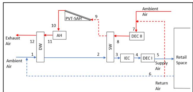
Figure 2: Schematic of Solar Assisted Desiccant Cooling System (DINC configuration)
