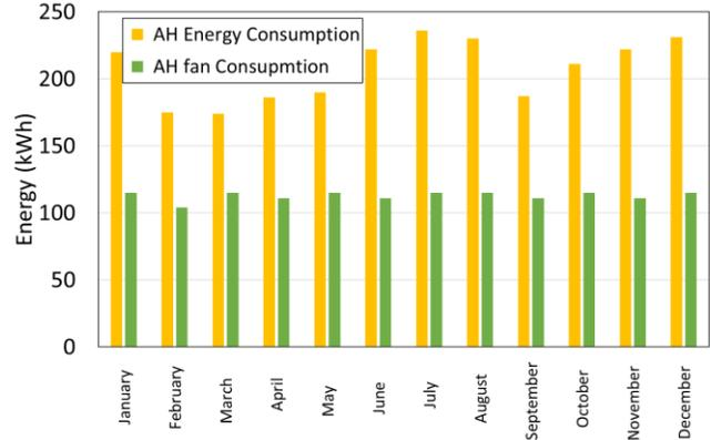
Figure 4: Monthly Energy profile of Auxiliary heater and fan consumption
