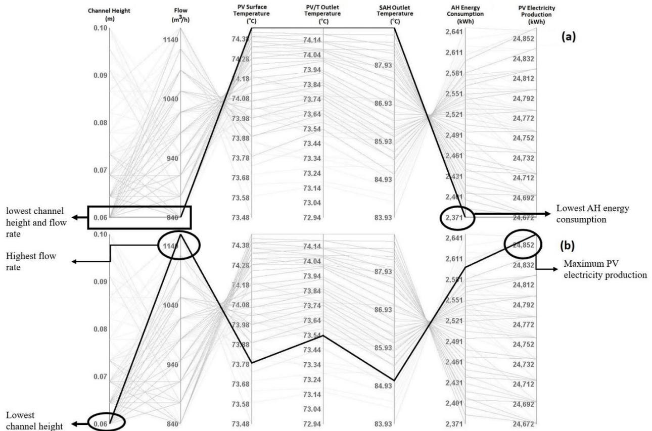
Figure 9: Parallel plots illustrating variation in outputs and present the configuration and the resulting performance with respect to (a) minimum AH energy consumption (b) maximum PV electricity production
