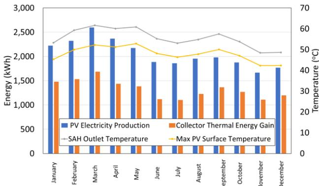
Figure 3: Monthly Energy Profile of PV/T+SAH subsystem
