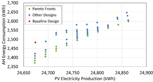
Figure 7. Optimization results of maximizing PV electricity production and minimizing AH energy consumption
