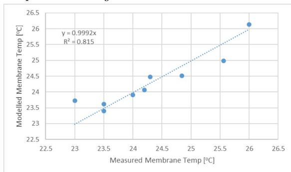
Figure 7: Correlation between modelled and measured membrane Temperatures after applying error factors.
