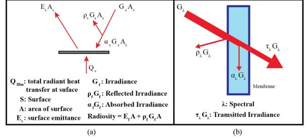
Figure 3: (a) Emission and irradiation on an opaque surface (b) Irradiation on a translucent surface
