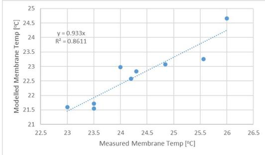
Figure 5: Correlation between modelled and measured membrane temperatures using Non-calibrated model.
