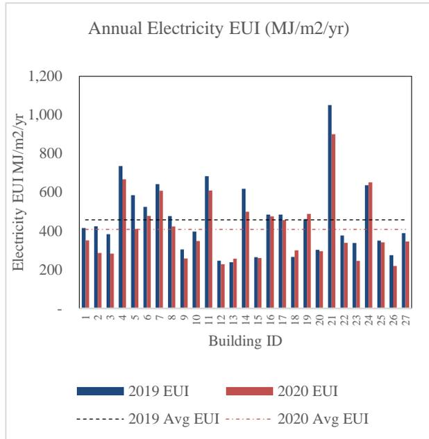
Figure 1: Annual electricity usage intensity for 2019 and 2020.
