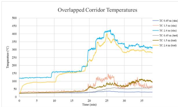
Figure 5. Comparisons of the simulated temperature and the measured temperature in the corridor (TC stands for thermocouple and the adjacent number shows its measurement height)
