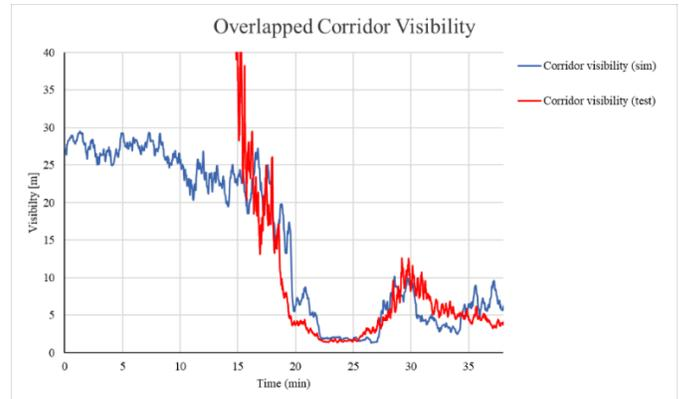
Figure 8. Comparisons of the simulation and test results for visibility in the corridor (at 1.5 m) (Note: FDS uses 30 m as the highest visibility for ambient condition)
