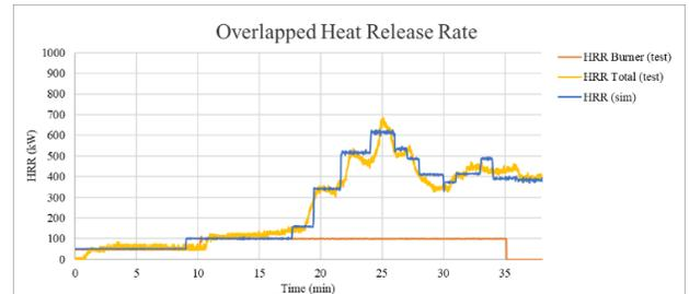
Figure 4. Comparisons of the simulation and test results for Heat Release Rate
