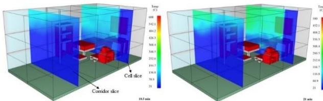
Figure 6. 2D temperature slices in the room and corridor at 18.5 and 21 minutes
