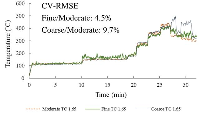
Figure 3. Grid independency test: temperature at a height of 1.65 m in the room for the simulations with the three different grid sizes
