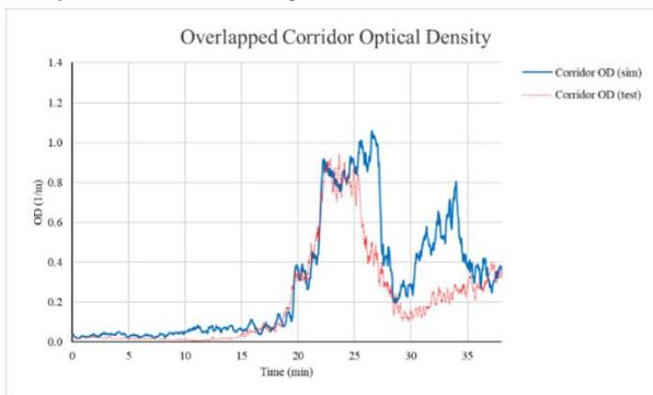
Figure 7. Comparisons of the optical density results from the simulation and the test (at 1.5 m)
