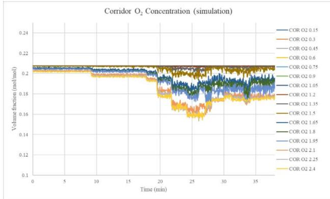
Figure 10. Simulated corridor  $O_2$  concentration along height (the numbers in the legend show oxygen sensor height in the corridor)
