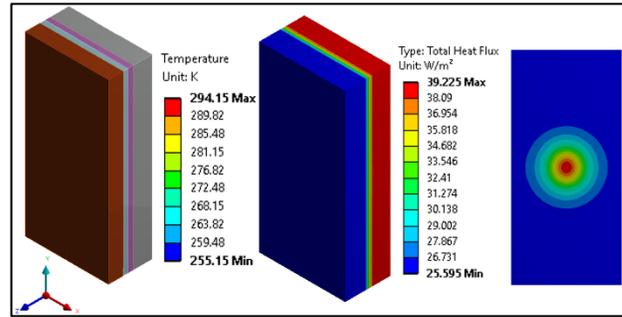
Figure 8: Thermal distribution and the heat flux for one-studied case of models type A
