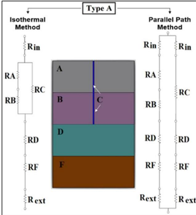
Figure 4: Equivalent isothermal and parallel thermal circuit for Type A assemblies (Note:  $R_{in}$  and  $R_{ext}$  are the interior and exterior air film resistance)
