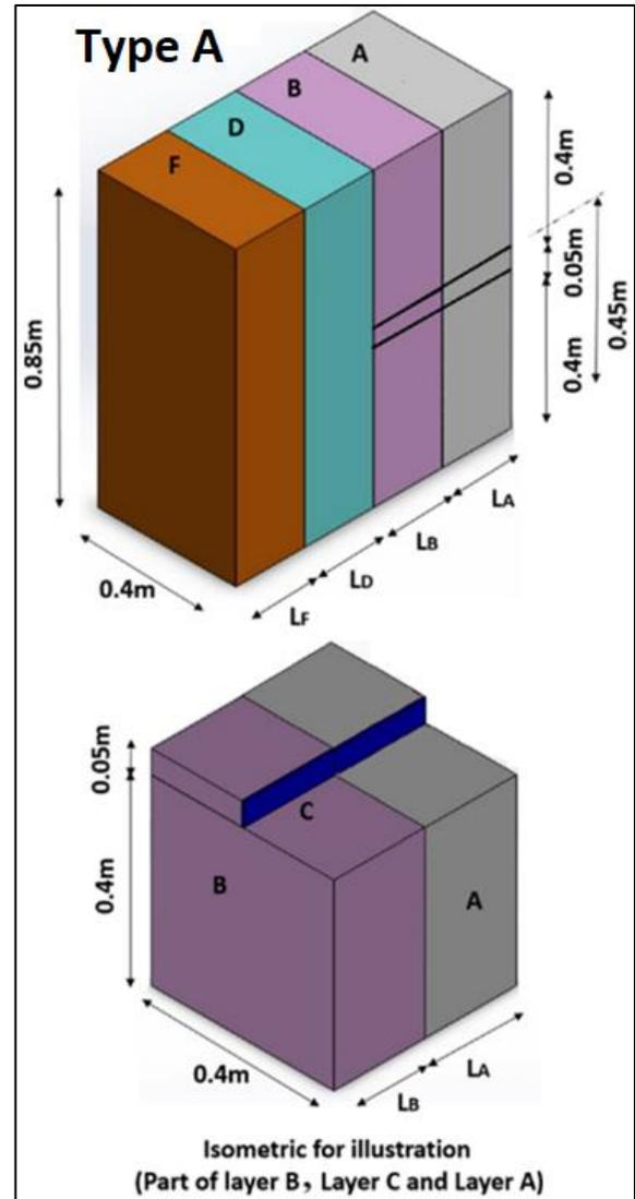
Figure 3: Simplified assemblies, Type A representing block tie type
