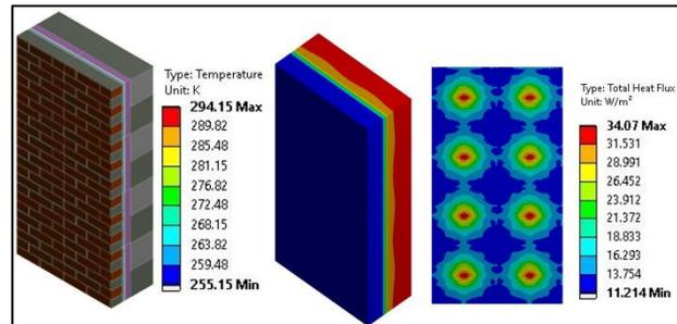
Figure 10: Thermal distribution and the heat flux for one-studied case of models type B
