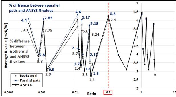
Figure 7: R-value results using isothermal, parallel path and ANSYS with respect to the Ratio
