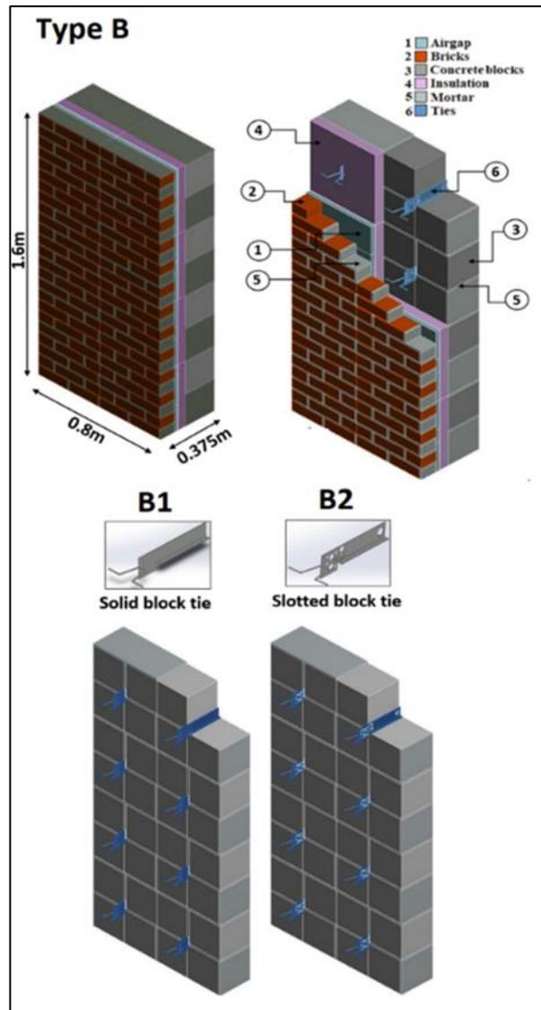
Figure 5: Detailed assemblies, Type B<sub>1</sub> and B<sub>2</sub> - Note: Since the walls' geometry is symmetrical, the geometrical complexity of the model was reduced by simulating only one tie and simplifying the total dimensions of the simulated model to be (400 X 400 X 375mm)
