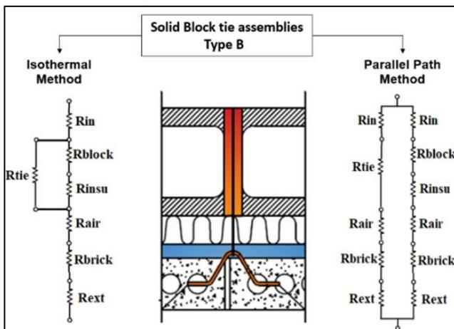
Figure 6: Equivalent isothermal and parallel thermal circuits for Type B assemblies (Note:  $R_{in}$  and  $R_{ext}$  are the interior and exterior air film resistance)
