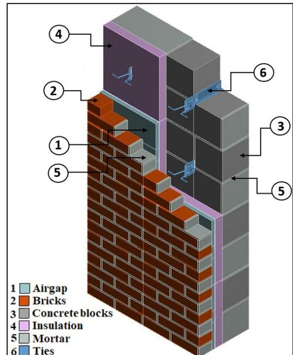
Figure 1: Components of clear masonry veneer walls
