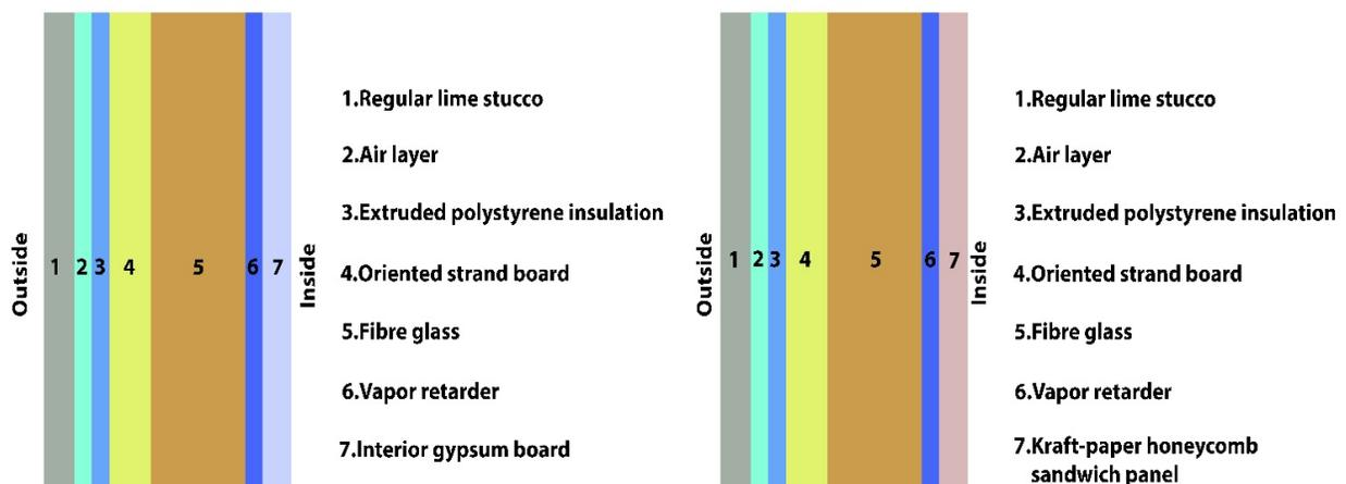
Figure 1. The composition of 1) reference wall 2) multilayer sandwich panel for numerical modelling.
