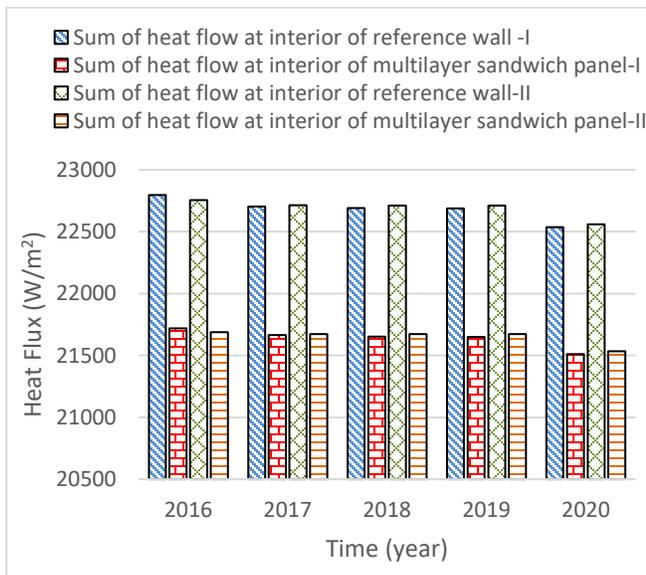
Figure 5. Annual heat flow of interior surface of the reference wall and multilayer sandwich panel under scenarios I and II.
