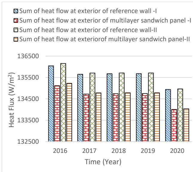
Figure 4. Annual heat flow of exterior surface of the reference case and multilayer sandwich panel under scenarios I and II.
