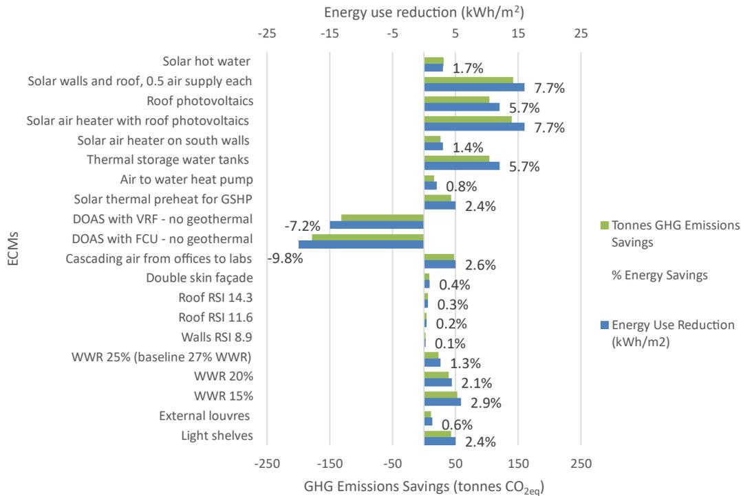
Figure 8: New laboratory additional individual energy conservation measures results. Energy savings and GHG emissions savings relative to baseline (203 kWh/m<sup>2</sup>, 1833 tonnes CO<sub>2eq</sub>).
