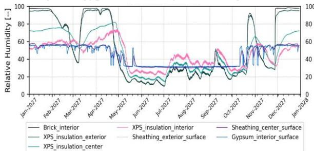
Figure 11: Design wall RH for all monitor points in the wall assembly within WUFI.
