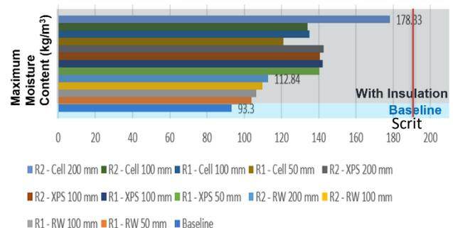
Figure 2: Different retrofit scenario moisture content results for the rubble stone layer (Scrit for concrete rubble stone is 189 kg/m<sup>3</sup>). Cell = cellulose, RW = mineral wool, XPS = extruded polystyrene. R# denotes retrofit scenario number.
