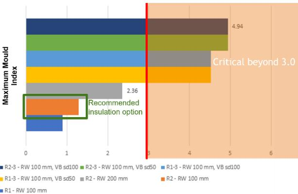
Figure 4: Maximum mould index for insulation with and without a vapour barrier on the interior side of insulation. R1 – add insulation on interior of existing wall. R2 – remove inner masonry, add insulation on interior side.
