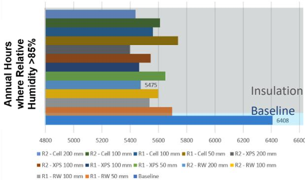
Figure 3: Annual hours where relative humidity is greater than critical level of 85% in the rubble stone core layer.
