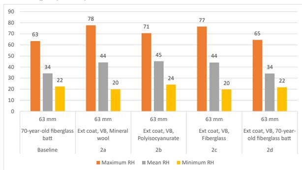
Figure 13: Maximum, mean, and minimum RH for insulation layer in the baseline and retrofit scenarios analysed.
