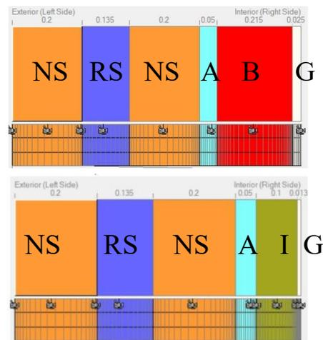
Figure 1: Baseline existing wall type 2 (top) and Retrofit 2 (bottom) wall compositions and monitor points (indicated by grey camera icons). NS – Nepean sandstone, RS – rubble stone, A – air gap, B – brick, G – gypsum board, I – insulation.
