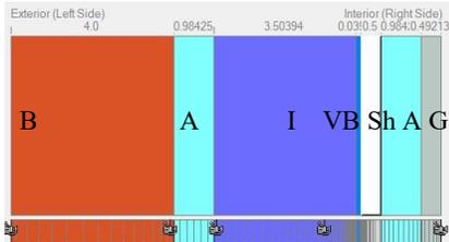
Figure 10: Design wall composition and monitor positions. See nomenclature for layer material names. B – brick, A – air gap, I – insulation, VB – vapour barrier, Sh – sheathing, G – gypsum board.
