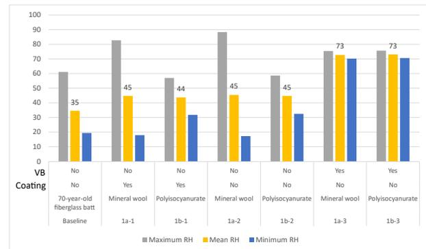
Figure 14: Maximum, mean, and minimum RH for concrete layer in baseline and 50 mm insulation scenarios with different combinations of either including or excluding the exterior coating and vapour barrier.
