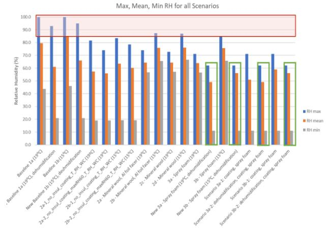
Figure 8: Max, mean, and min RH at the interior surface of wall assembly for all scenarios simulated.
