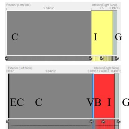
Figure 12: Baseline existing wall (top) and Retrofit (bottom) and monitor positions. C – concrete, I – insulation, G – gypsum, EC – elastomeric coating, VB – vapour barrier.
