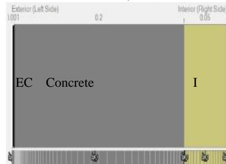
Figure 5: Retrofit with exterior coating and insulation and monitor points (indicated by grey camera icons). EC – elastomeric coating, I - insulation.
