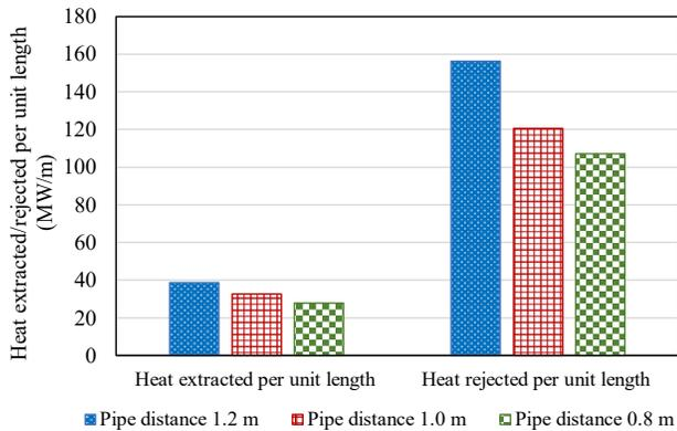
Figure 4. Annual heat extracted/rejected by the GHE per unit length (1 m depth)
