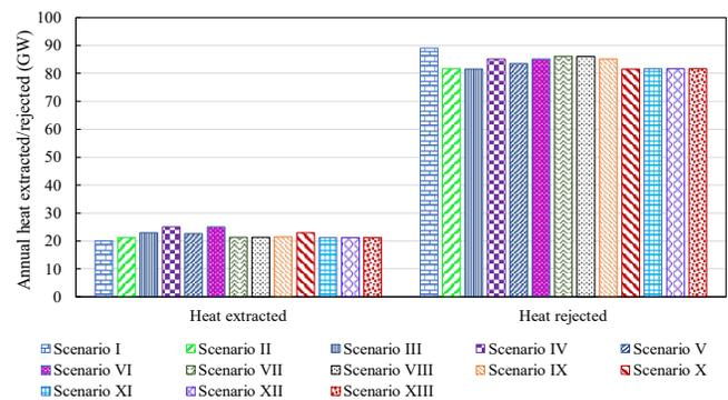
Figure 3. Annual heat extracted/rejected by the GHE
