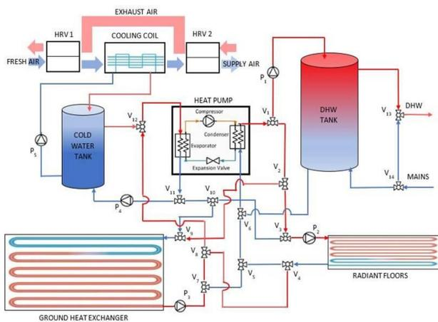
Figure 1. System configuration
