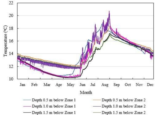
Figure 6. Annual variation of soil temperature under Zone 1 (end zone) and Zone 2 (middle zone)
