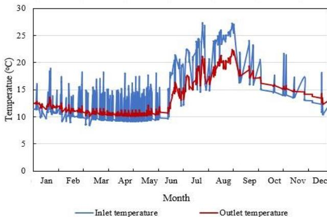
Figure 5. Annual variation of the GHE inlet and outlet temperature
