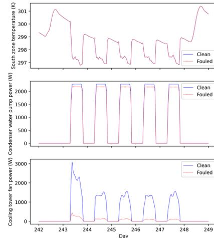
Figure 2 Performance comparison between clean (case 0) and fouled (case 4) conditions for south zone temperature, condenser water pump power, and cooling tower fan power in a typical summer week (Aug. 30<sup>th</sup> – Sep. 6<sup>th</sup>).
