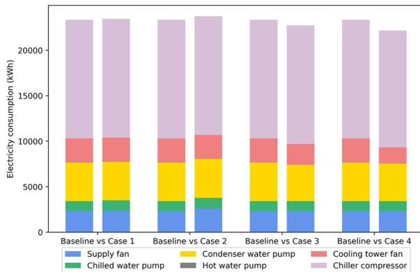
Figure 3 Electricity consumption by end use for baseline and all faulty cases.
