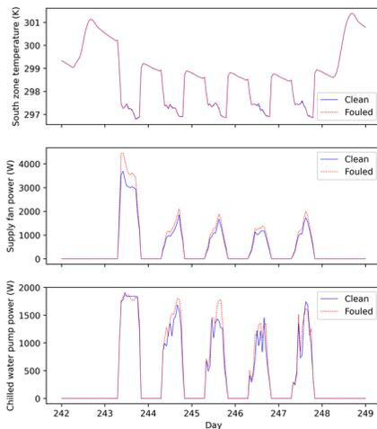
Figure 1 Performance comparison between clean (case 0) and fouled (case 2) conditions for south zone temperature, supply fan power, and chilled water pump power in a typical summer week (Aug. 30<sup>th</sup> – Sep. 6<sup>th</sup>).
