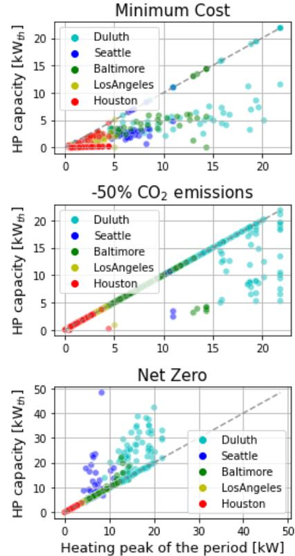
Figure 8: Relation between peak heating load and HP capacity in residential buildings.
