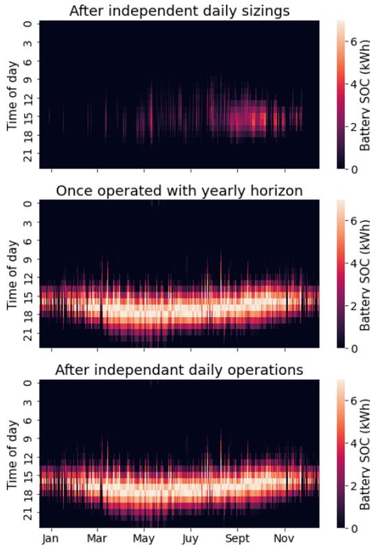
Figure 5: Example of the expected usage of a battery right after the sizing step (top), then after operating the so sized system with horizons of a year (middle) and a day (bottom) in Baltimore (MD).
