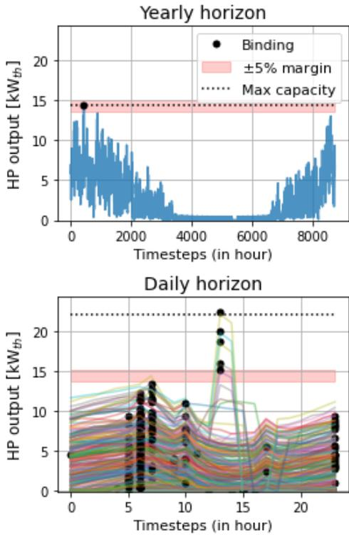
Figure 7: Location of binding constraints for HP capacity sizing in Baltimore for net-zero residential building.
