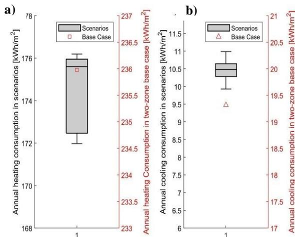
Figure 7. Annual heating (a) and cooling (b) consumption comparison between the two-zone base case and scenarios.
