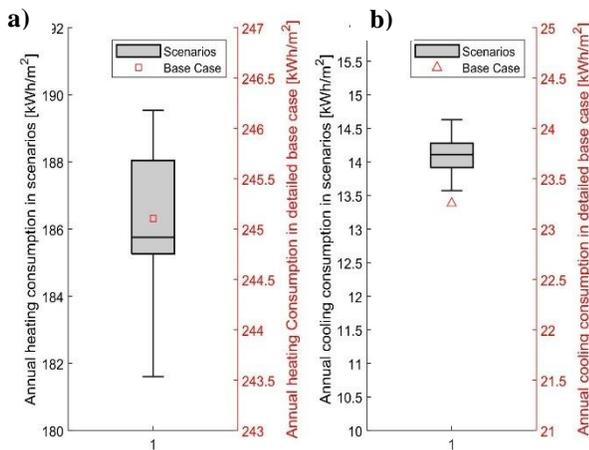
Figure 6. Annual heating (a) and cooling (b) consumption comparison between the detailed base case and scenarios.
