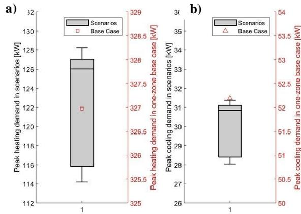
Figure 11. Peak heating (a) and cooling (b) demand comparison between the one-zone base case and scenarios.
