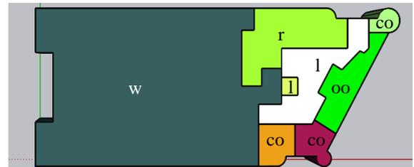
Figure 3. Thermal zones in the base model: Warehouse (w), Closed Office (co), Open Office (oo), Lobby (l) and Restroom (r).
