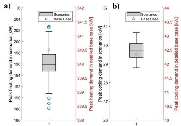
Figure 9. Peak heating (a) and cooling (b) demand comparison between the detailed base case and scenarios.
