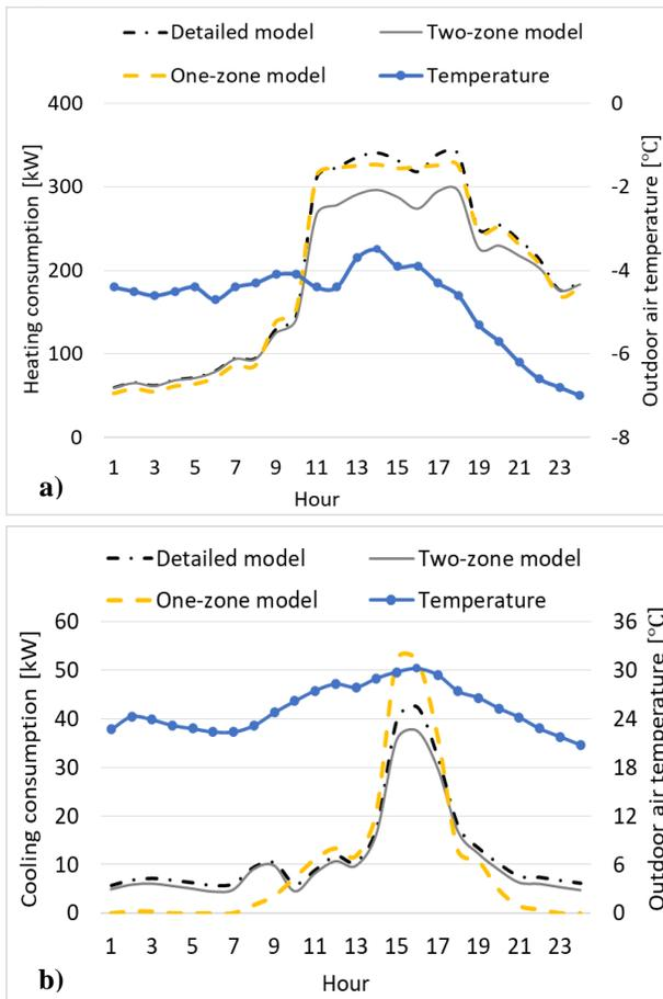
Figure 12. Hourly heating (a) and cooling (b) energy consumption on February 27<sup>th</sup> and July 21<sup>st</sup>, respectively.
