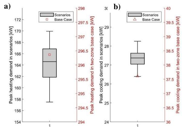
Figure 10. Peak heating (a) and cooling (b) demand comparison between the two-zone base case and scenarios.
