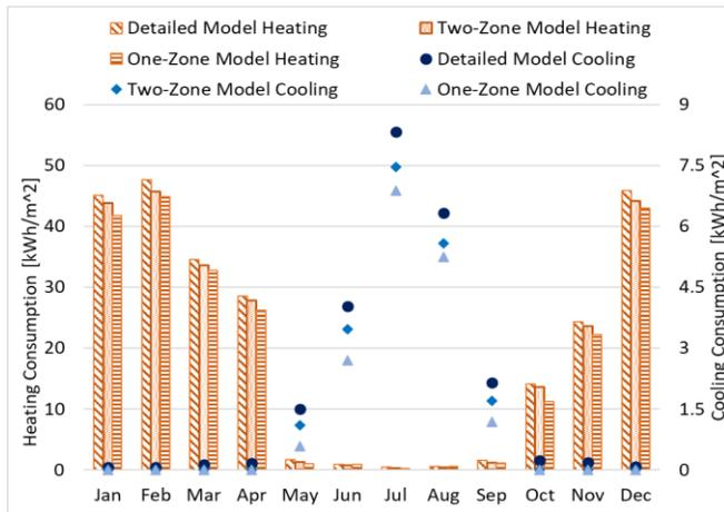
Figure 5. Monthly heating and cooling consumption in detailed and simplified models.
