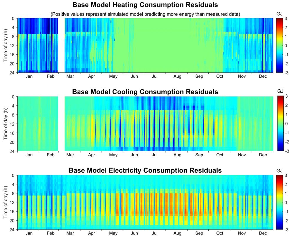
Figure 3: Base model energy map of the differences between simulated data and measured data. Blank sections depict missing utility data.
