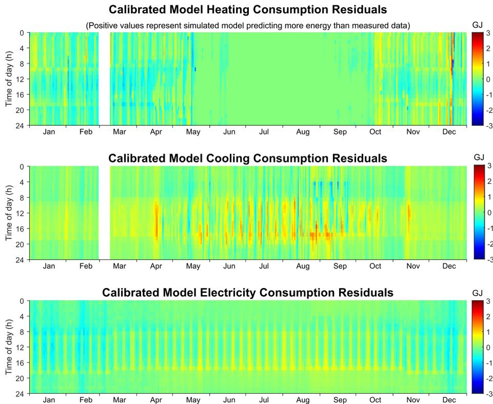
Figure 4: Calibrated model energy map of the differences between simulated data and measured data. Blank sections depict missing utility data.
