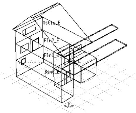
Figure 2. ESP-r model of the west unit of the CCHT facility.
