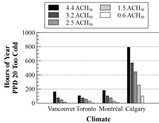
Figure 10. Fraction of year 20% PPD too cold on second floor.
