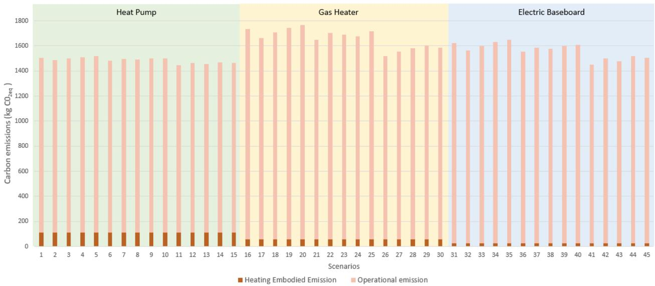
Figure 9- The impact of heating system on embodied and operational emission
